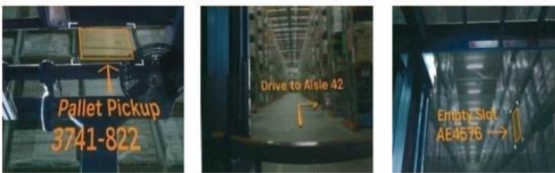
Figure 9: The left image shows which object that should be picked. The middle image illustrates the recommended route for navigating within the warehouse. The right image represents the destination where the object should be placed [Pereira et al. 2016]
