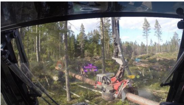
Figure 11: The image shows the view from the cabin operator's position when doing the cutting operation. The operator is supported by information from the bucking optimization system presented on a head-up display, seen in pink in the middle of the image [Englund et al. 2015]
