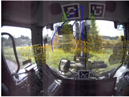
Figure 2: The blue line represents the crane's structure, while the point clouds represent the environment in front of the machine [Palonen et al. 2017]
