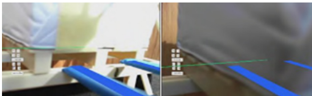
Figure 3: The left image shows blue virtual quads that represent the position of the forks. The right image shows a green line that indicates the maximum depth, where the forks can be moved to [Sarupuri et al. 2016]
