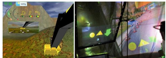
Figure 10: The left image shows instrumentation-related information that is presented near the line of sight [Akyeampong et al. 2014]. The right image shows navigational information and obstacle warning that are also presented near the line of sight [Wallmyr et al. 2018]
