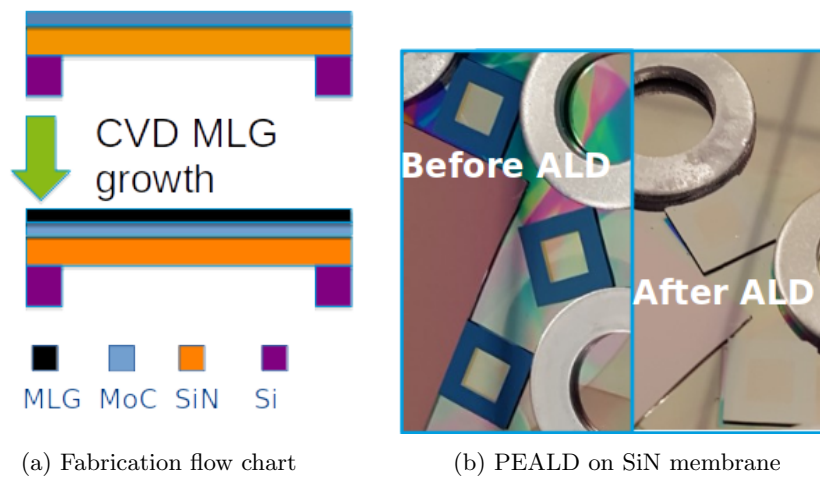
Figure 4: Illustration of suspended heterostructure and optical images. Left (a) Fabrication schematics of suspended graphene heterostructure. (b) Right: Optical images of SiN membranes before and after PEALD of \sim 15 nm MoC_x film on top.
