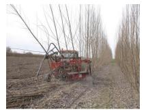
Figure 16.5 – cut- windrower for small plants (2 years old)
