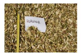
Figure 17.4 – chips produced with the Class jaguar 880
