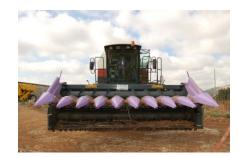
Figura 14.6 – CRESSONI bit3g header specifically designed for cardoon
