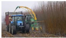
Figure 18.2 – tractor mounted maize header use on SRC
