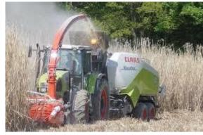
Figure 6.4 – tractor mounted Maize silage harvester utilized on miscanthus with unload directly in the square baler
