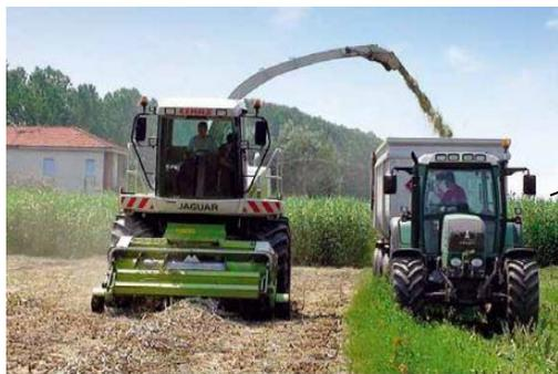
Figure 7.5 - System 3: Claas Jaguar 850 and PU 300 HD
