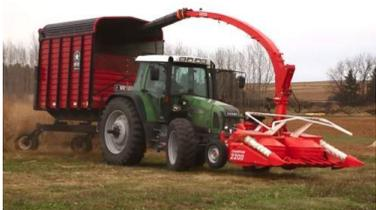
Figure 5.5 – tractor mounted maize silage harvester and trailer
