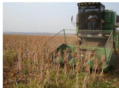
Figure 4.3 – Maize header used for castor bean
