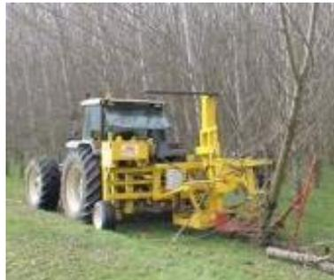
Figure 16.7 – cut windrower for large plants (5 years old)
