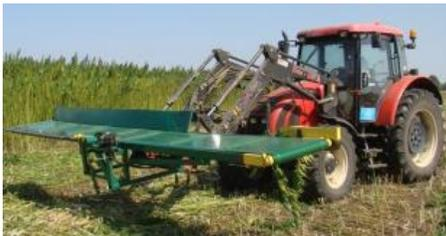
Figure 10.7 - Cutting bar with belt for the transport of the panicles
