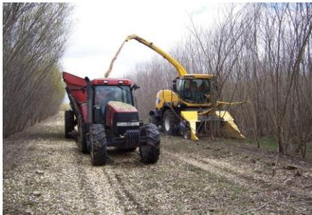
Figure 18.3 – self propelled forage harvester equipped with SRC header
