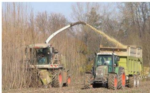
Figure 16.2 – single pass, cut and chip method
