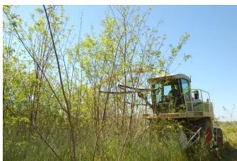
Figure 17.2 – cut and chipping with Claas jaguar 880 and GBE1 header
