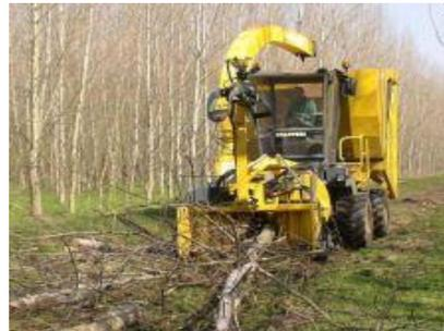
Figure 16.8 – pick up chipper for large plants (5 years old)
