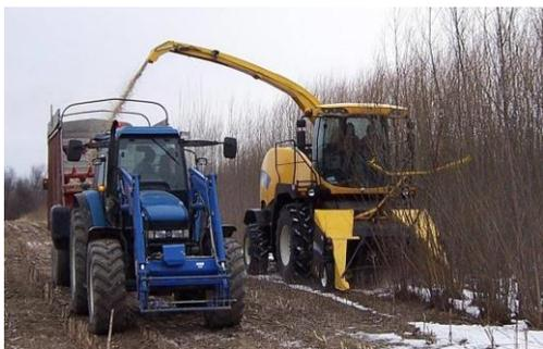
Figure 15.3 – cut and chip method
