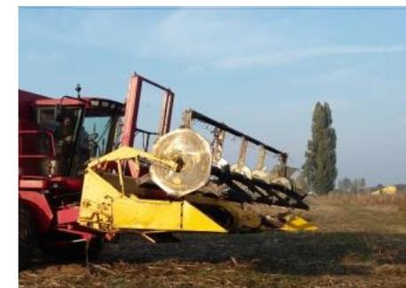
Figure 10.4 - Modified combine with elevation system for wheat header
