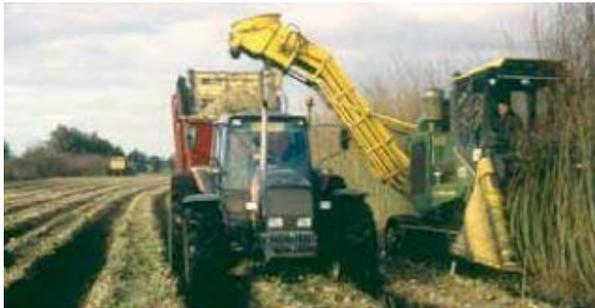
Figure 15.4 – cut and billet method
