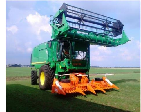
Figure 10.6 - Double cut system
