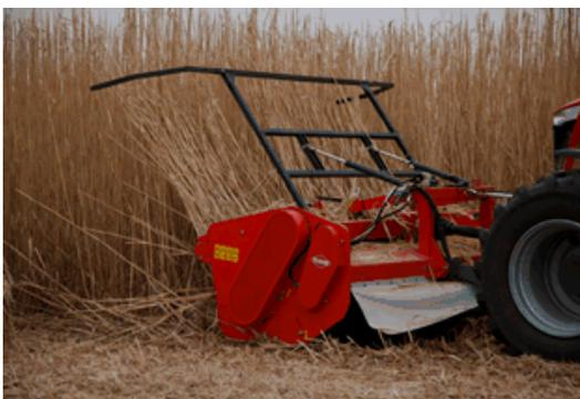
Figure 6.2 – shredder attached to the front PTO of the tractor
