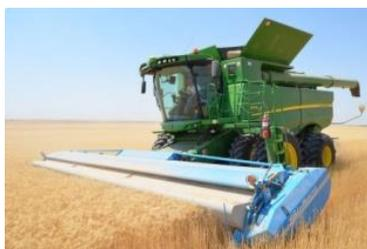
Figure 2.3 – header with stripping rotor
