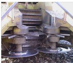
Figure 16.3 – header GBE for the cut and chip method
