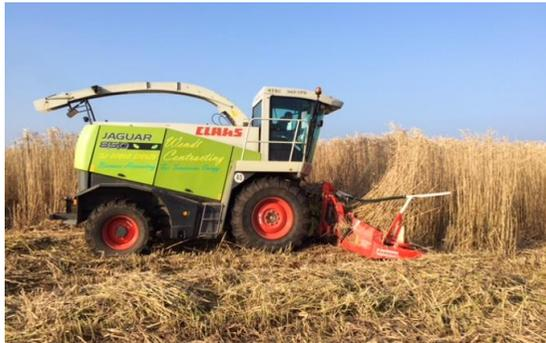
Figure 6.3 – class jaguar with keper type header working on miscanthus
