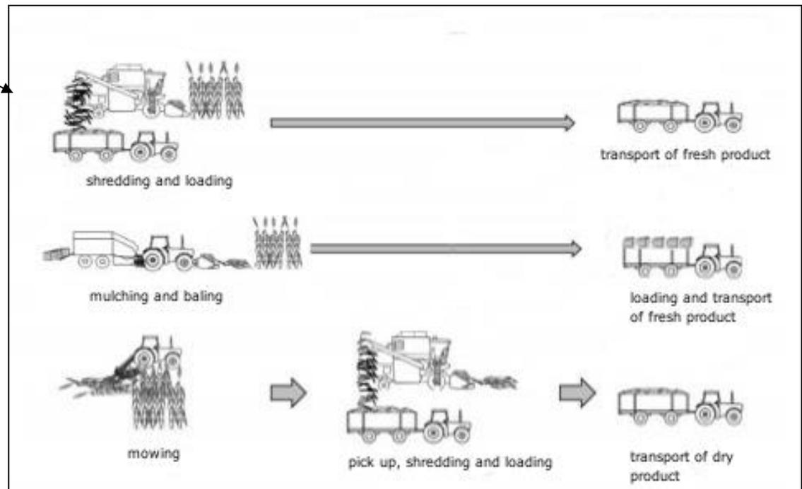
Figure 7.5 – scheme of the three harvest systems for arundo
