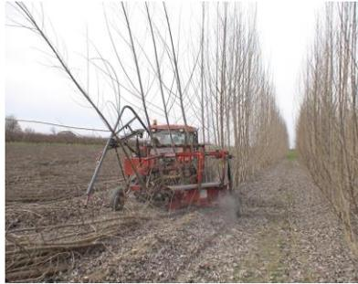
Figure 16.5 – cut- windrower for small plants (2 years old)
