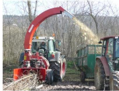
Figure 16.6 – pick-up chipper for small plants (2 years old)
