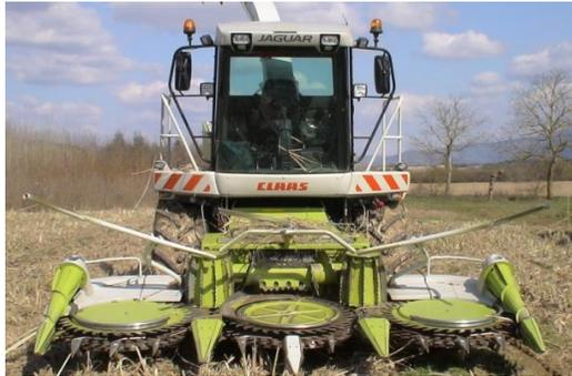
Figure 1.3 – Class Jaguar SPFH with kemper type header
