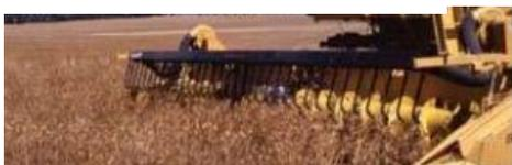
Figure 20.3 – traditional reel replaced with air reel
