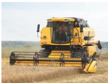
Figure 3.3 – combine with header for wheat used for crambe
