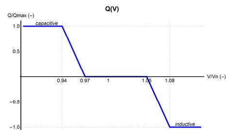
Figure 1. Autonomous Q (V) function of smart PV inverter
