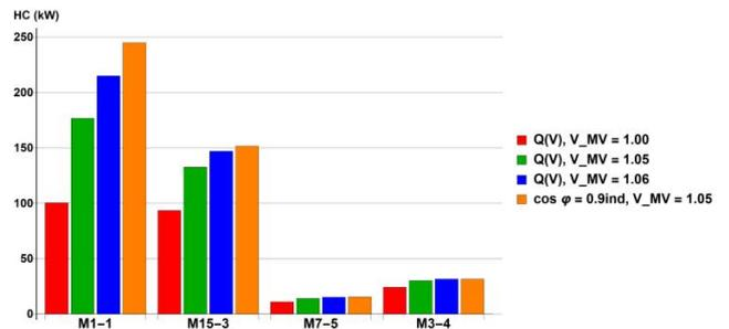
Figure 8. Hosting capacity results for representative feeders
