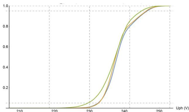
Figure 14. Monthly distribution function for PV phase-to-ground voltages
