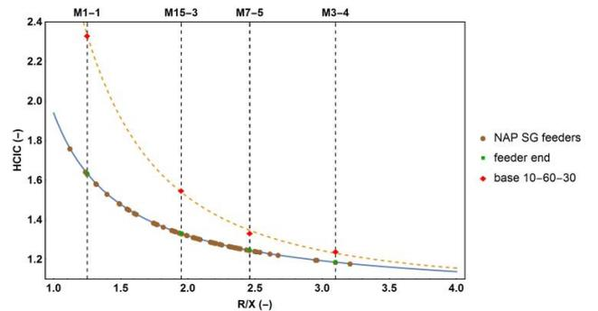
Figure 4. Hosting capacity increase by means of DER reactive power (power factor = 0.9, inductive mode) and DER placement
