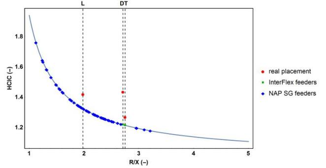
Figure 3. Hosting capacity increase by means of DER reactive power (power factor = 0.9, inductive mode)
