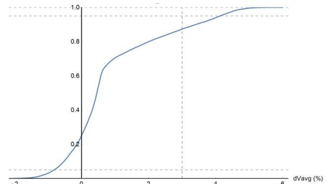
Figure 13. Monthly distribution function for voltage difference between transformer and PV (feeder end)
