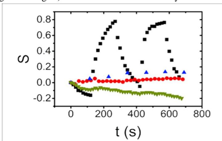
**Figure S3. Control experiments.** Relative signal variations,  $S$ , of the proposed LEGOT (black squares), LEGOT with randomly oriented RC on the Gate (red dots), control EGOTs featuring a bare ITO Gate (blue triangles) and a cyt  $c$ -functionalized ITO Gate (green triangles).
