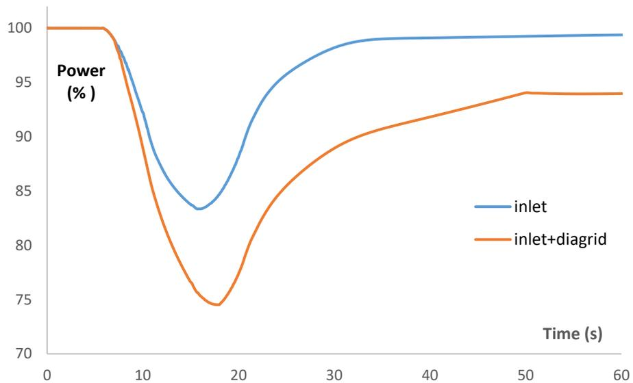
Figure 5. Power evolution during the transient accounting for diagrid expansion
