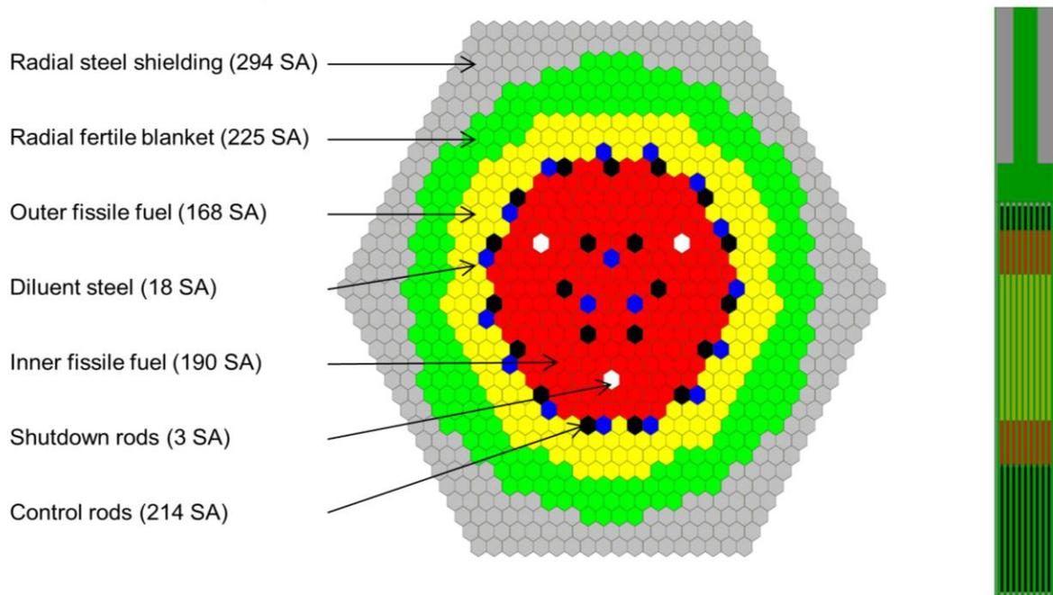
**Figure 1. Top view of the SERPENT benchmark model of SPX (left) and side view of a fuel SA (right)**
