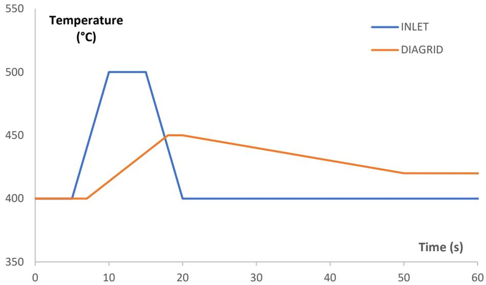
Figure 4. Diagrid and core inlet temperature evolutions during the transient
