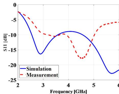
Fig. 7. Measured and simulated reflection coefficient results of on-body antenna on the muscle phantom.
