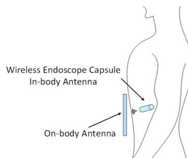
Fig. 1. The diagram of Wireless Endoscope Capsule communication.
