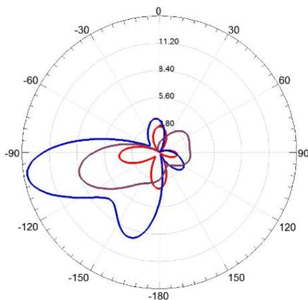
Fig. 4. Simulated radiation patterns ( $\phi = 90$  deg) of the in-body antenna at 3 GHz, 4 GHz and 5GHz inside the muscle phantom.
