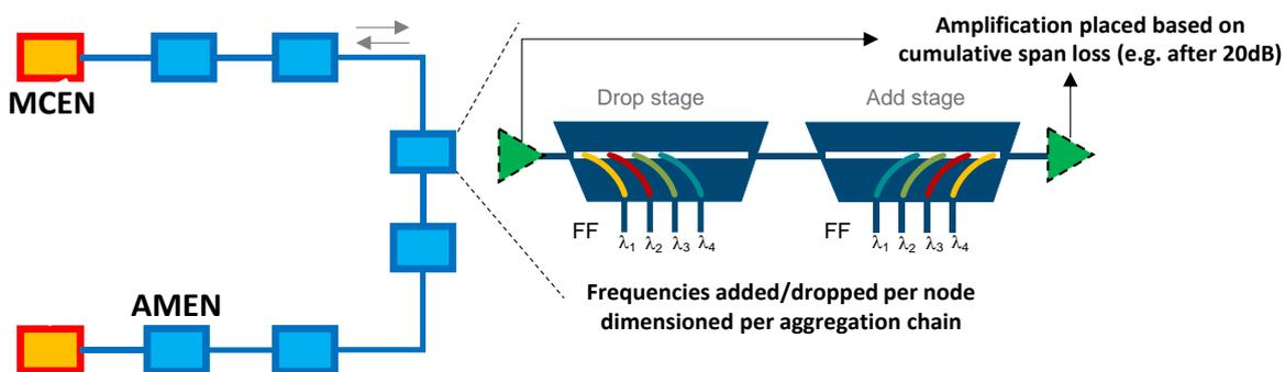
Figure 30: Fixed-frequency filter based express architecture.
