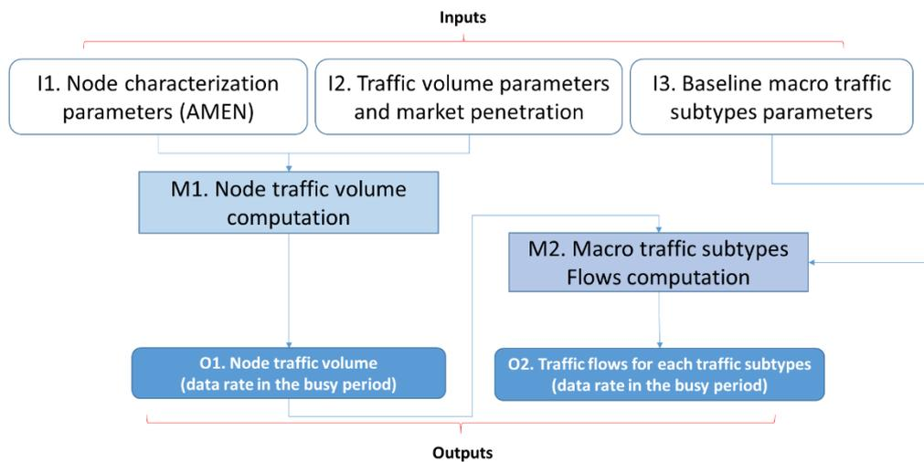
Figure 9: Methodology to compute the traffic offered to the node and flows associated with subtypes for background mass-market traffic (type T1 of AMEN (UPF type 2).
