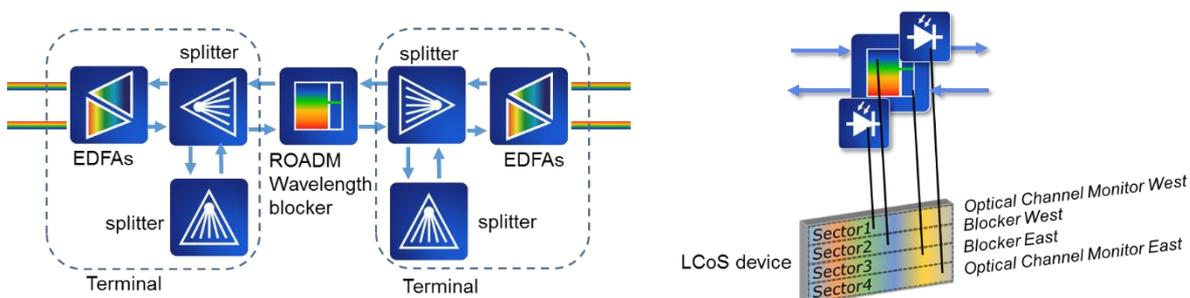
Figure 43: Left: ROADM node based on wavelength blocker, with terminals including amplifiers and splitters. Right: ROADM device with sectioned LCoS chip for blocking/power adjusting and monitoring functionality.
