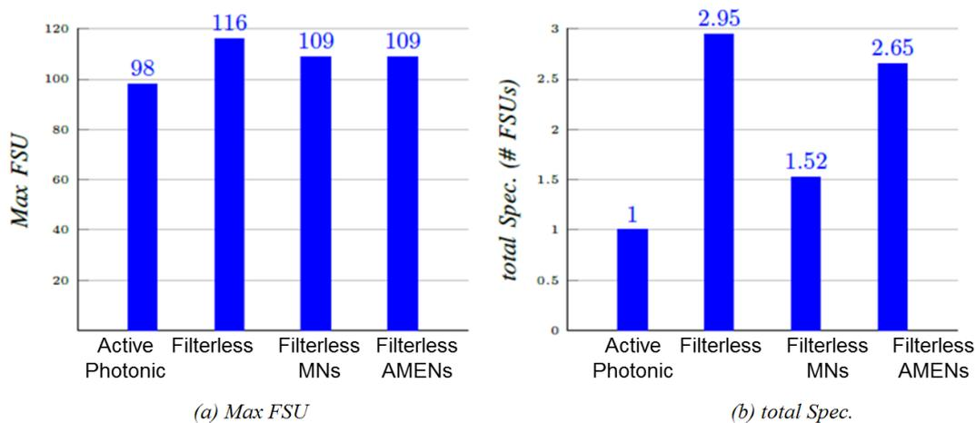
Figure 40: Comparison of the network deployments in terms of (a) Max FSU and (b) total Spec. (normalized to that of Active Photonic).
