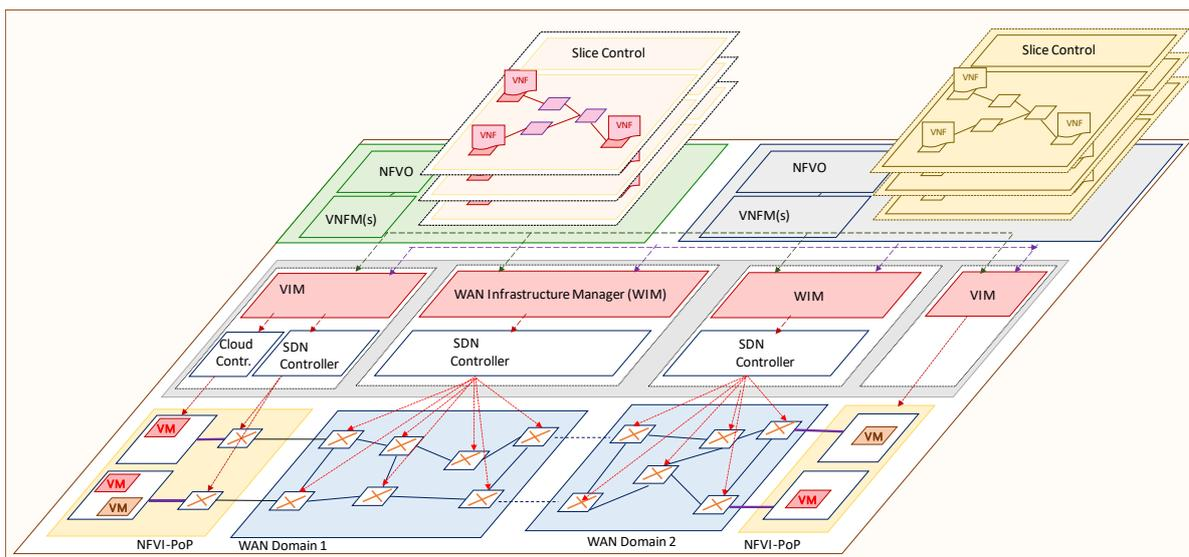
Figure 62: Network Slicing using the integrated SDN/NFV framework.
