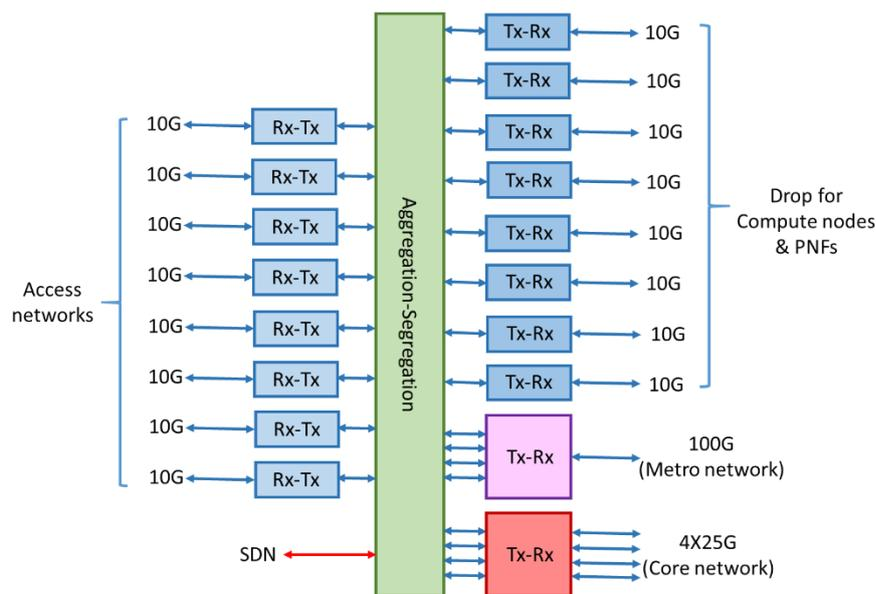
Figure 27: FPGA-based Programmable Switch Architecture
