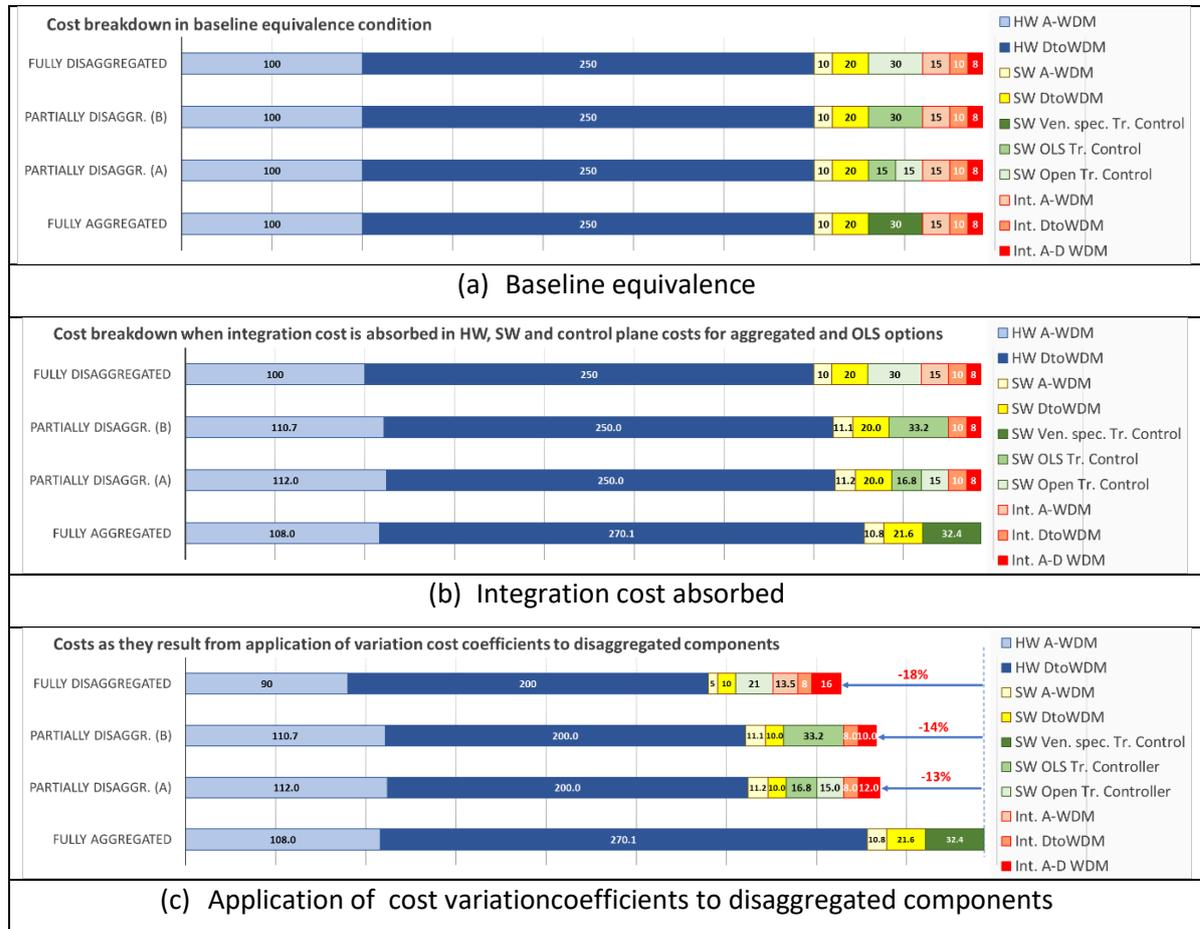
Figure 47. Cost breakdown of aggregated and disaggregated options under three different conditions.
