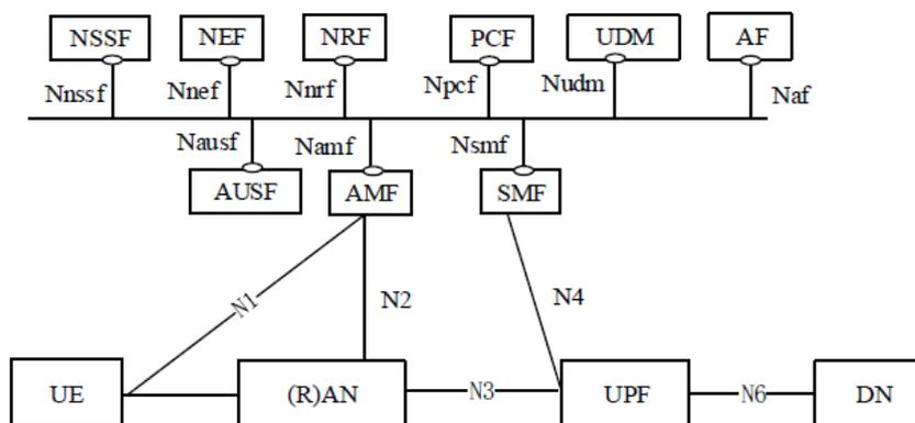
Figure 7: 5G System architecture interface representation (top: control plane, bottom: user plane) [3GPP-TS-22.261]
