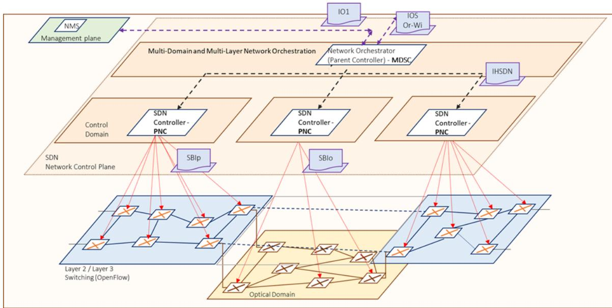
Figure 59: METRO-HAUL Network Control layer
