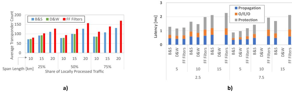
Figure 36: Evaluation of metro aggregation requirements per express architecture: a) transponders (10 node chain); b) latency.
