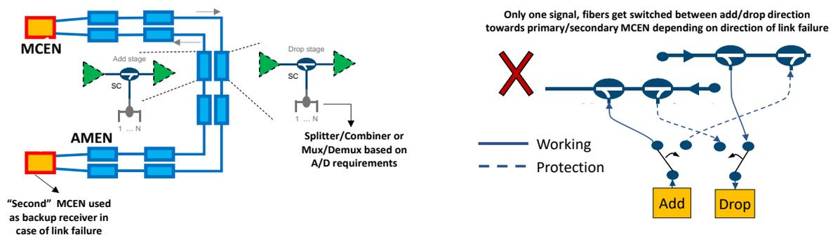
Figure 32: Filterless DuFiNet express architecture and protection requirements.
