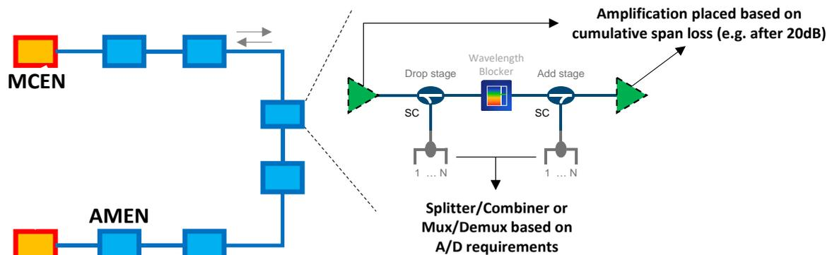
Figure 33: Semi-filterless wavelength-blocker based express architecture.
