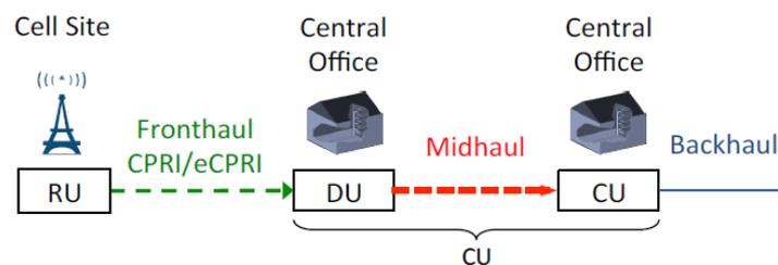
Figure 54: eNB functional separation in 5G networks. In this paper, we assume that the DU is co-located with its corresponding CU
