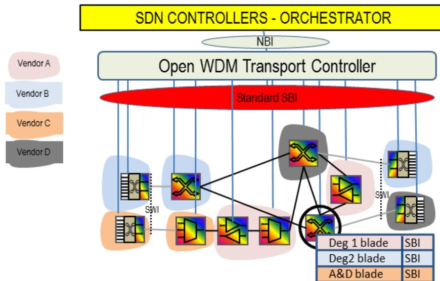
Figure 46. A fully disaggregated optical domain; figure 15 of D3.1)
