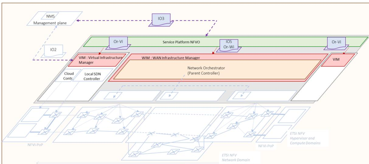
Figure 61: Metro-Haul Orchestration layer based on ETSI/NFV MANO
