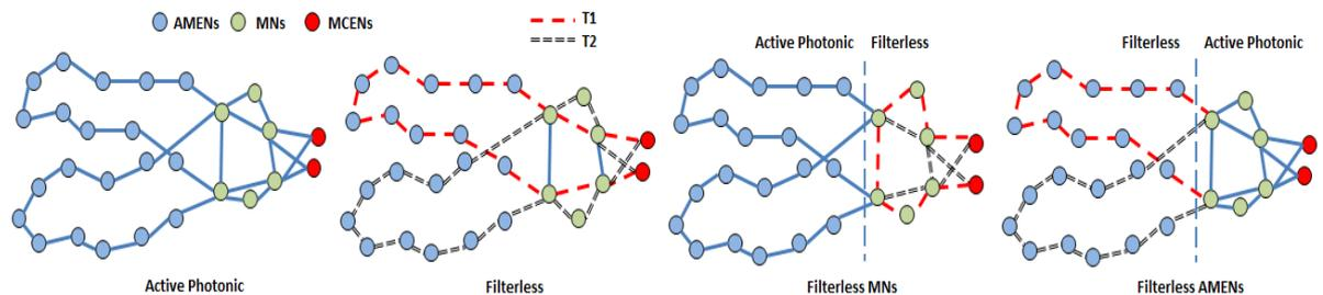
Figure 39 (From left to right) The network topology for the Active Photonic and the fiber tree formation for the Filterless, the Filterless MN and the Filterless AMENs. Note that the ANs are not sketched as they act as leaves and belong to the same fiber.
