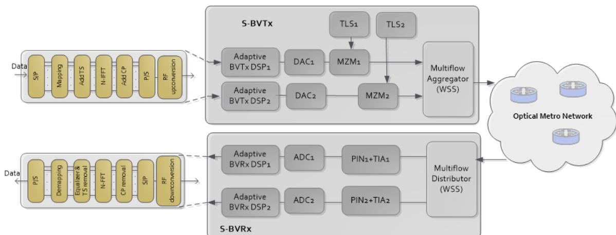
Figure 41. Programmable S-BVT architecture composed of two BVT modules based on MCM and DD.
