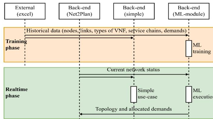
Figure 18: Workflow showing the integrated components that shows both the training and real-time phases.
