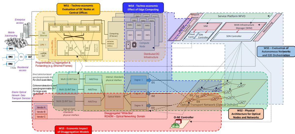
Figure 4: Mapping of working streams in the context of the Metro-Haul node and network architecture.
