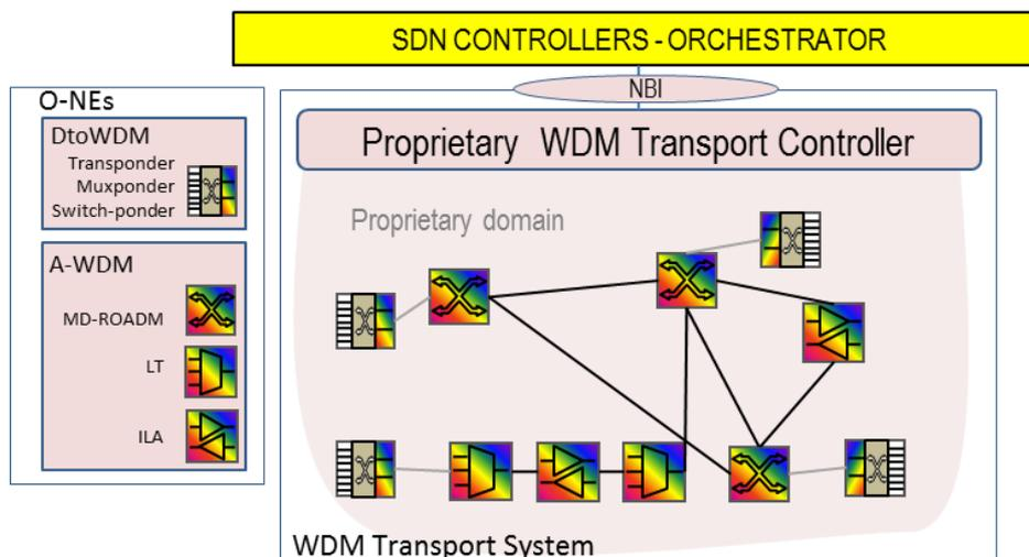
Figure 44. A fully aggregated optical network (figure 13 of D3.1)
