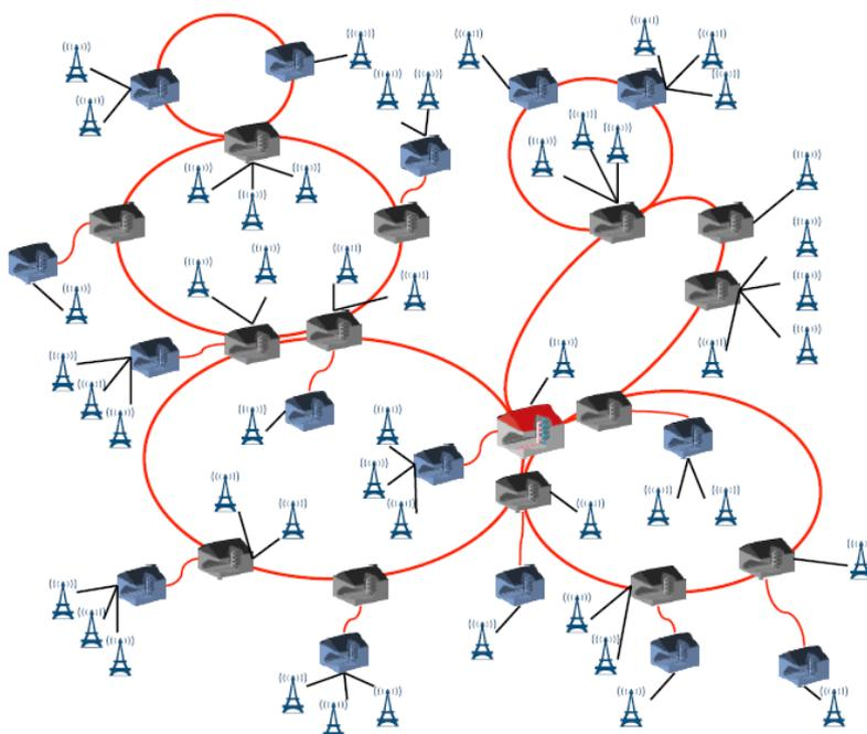
Figure 55 Hierarchical access-aggregation network architecture
