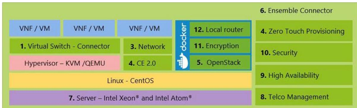
Figure 29: Compute Node Software Platform
