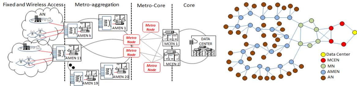
Figure 38: A schematic representation of the network topology showing the 4 network levels (left) and the network topology considered in our study (right).
