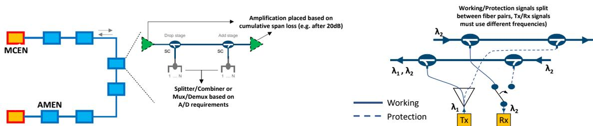
Figure 31: Filterless drop & waste express architecture and protection requirements.
