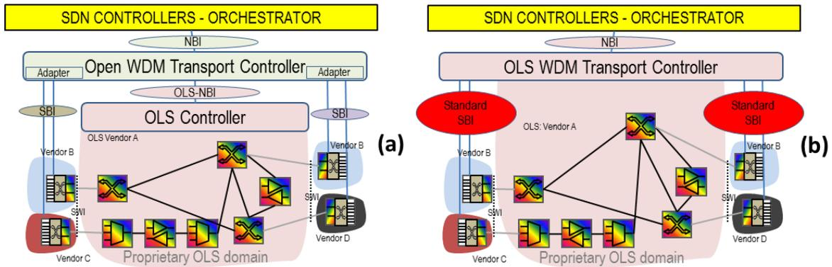
Figure 45. A partially aggregated optical network with (a) proprietary SBI, or (b) standard SBI; (figure 14 of D3.1)
