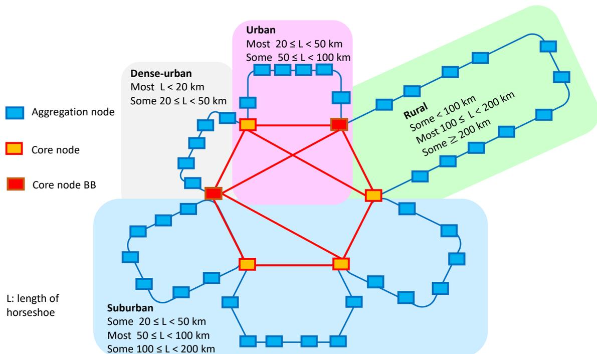
Figure 6. Reference Metro-Haul topology ( $L$  is the total horseshoe fiber length)
