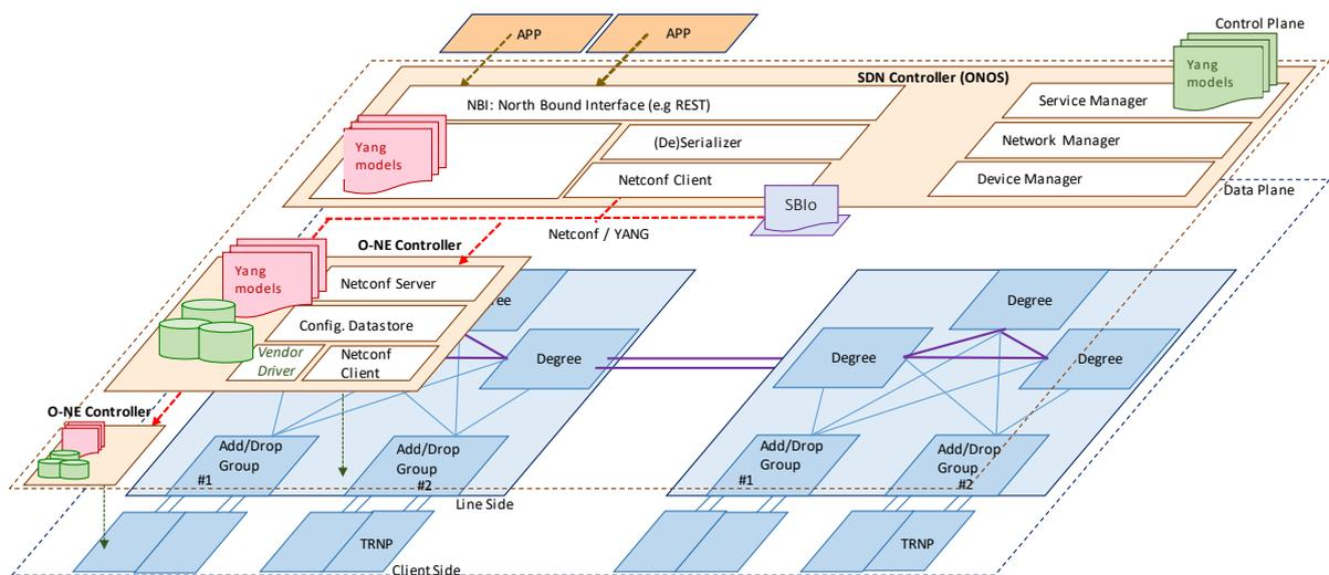
Figure 60: NETCONF / YANG control of the partially disaggregated optical network
