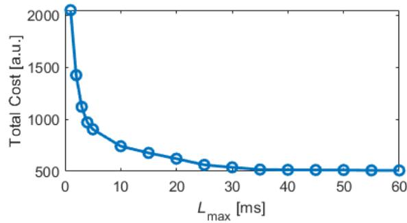
Figure 48: Total network cost as a function of the maximum latency allowed to reach the first VNF.
