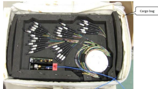
Figure 12: UV-VIS and fiber Switch in 0.5 CTB for vibration and shock tests
