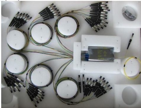
Figure 7: Optical Fiber Switch 1x48 channels
