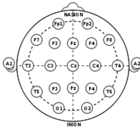
Figure 1: Diagram showing the 10-20 International System of Electrode Placement. The letters correspond to the regions of the cerebral cortical regions (Fp = frontal pole, C = central, P = parietal, O = occipital). Odd numbers correspond to the left hemisphere, and even numbers correspond to the right hemisphere.
