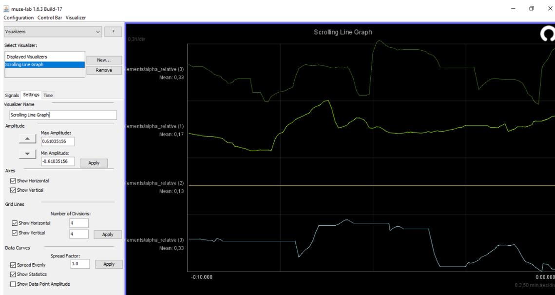
Figure 9: Screenshot of the MuseLab data visualizer showing live scrolling alpha absolute bandpower data.
