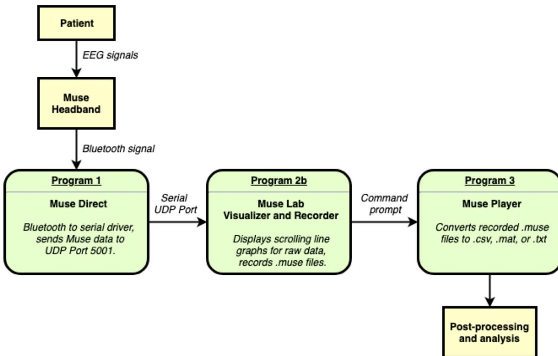
Figure 17: This chart shows the data flow sequence for the recording and post-processing and analysis of EEG activity.
