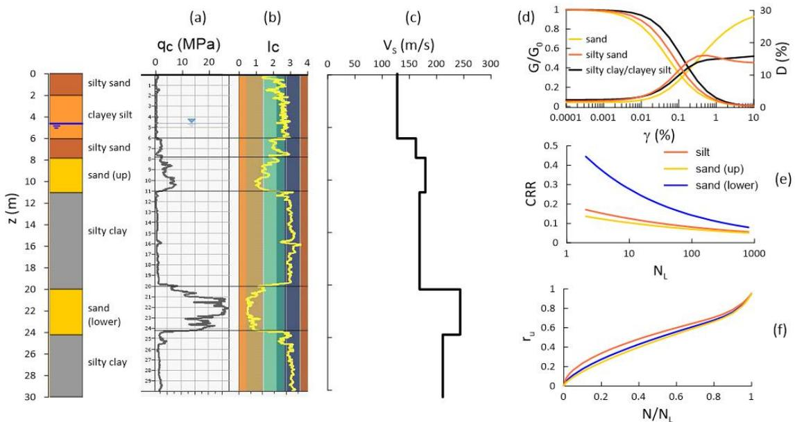
Figure 5. Vertical profile of cone tip resistance (a), soil behaviour type (b), shear wave velocity profile (c), shear modulus reduction and damping ratio curves (d), cyclic resistance (e) and excess pore water pressure ratio curves adopted in the model.
