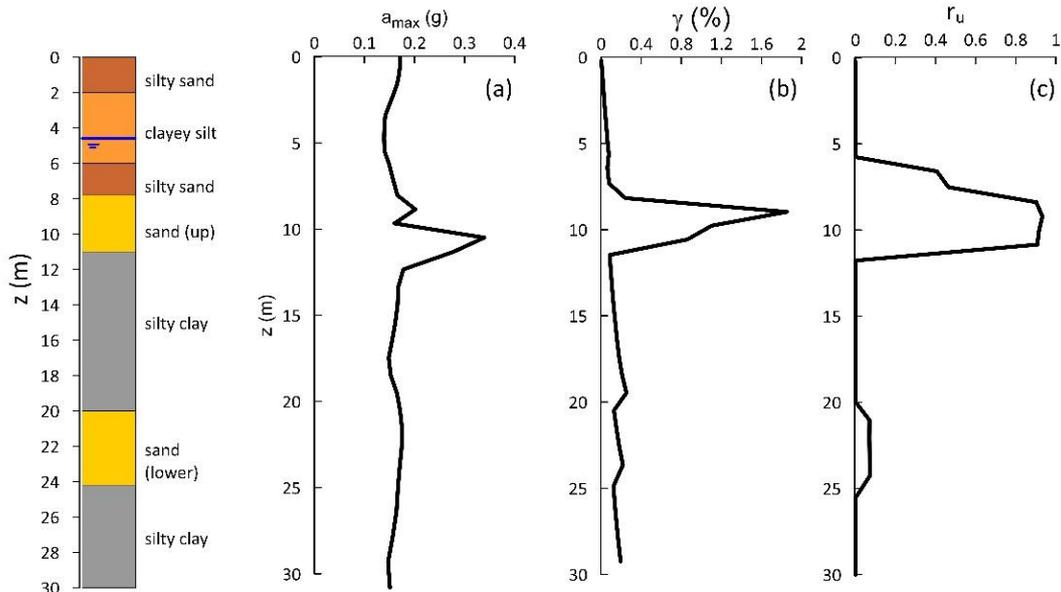
Figure 6. Results of the 1D dynamic analysis in terms of vertical profiles of maximum (a) acceleration, (b) shear strain and (d) pore pressure ratio.
