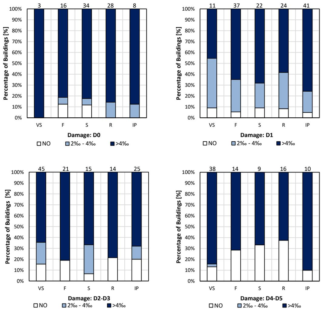
Figure 3. Percentage of buildings in function of levels damage defined to AeDES form.
