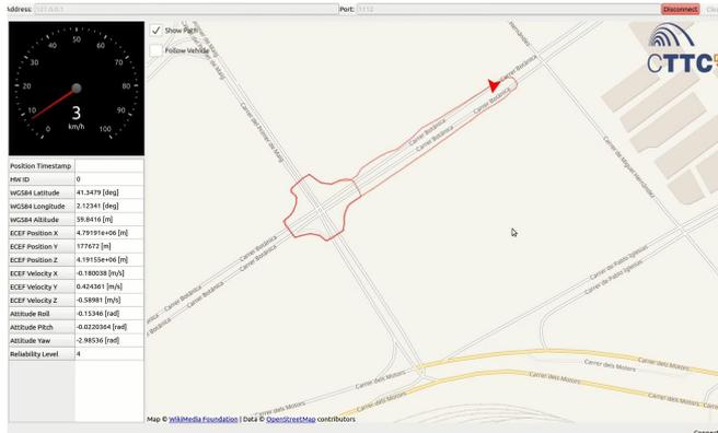
Fig. 8. Route followed by the bicycle resulting from the hybrid positioning algorithm.
