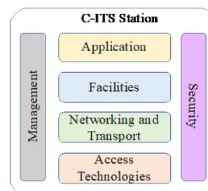
Fig. 2. C-ITS communication protocols architecture.
