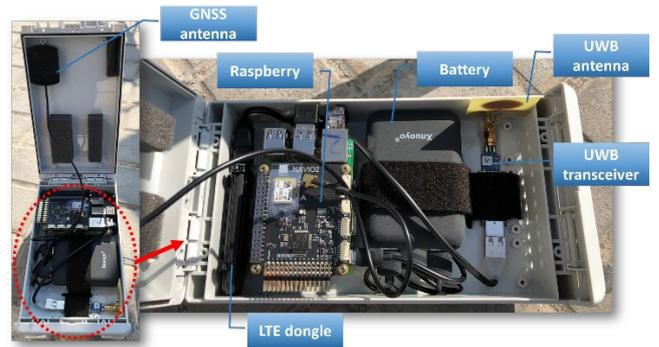
Fig. 3. Hybrid GNSS/INS/UWB positioning prototype.
