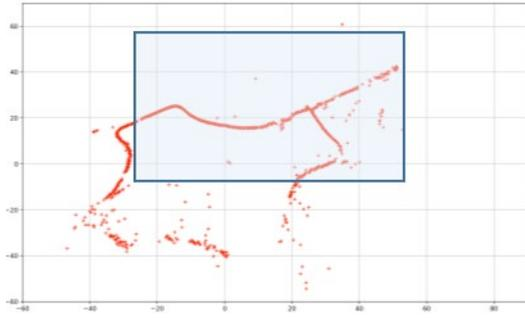
Fig. 12. Route followed by the bicycle using only UWB ranging triangulation.
