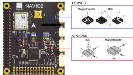
Fig. 4. Details of NAVIO2 IMU board (Emlid Ltd).
