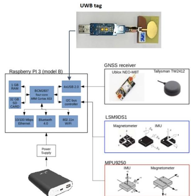
Fig. 5. Schematic fusion prototype inputs and interfaces.
