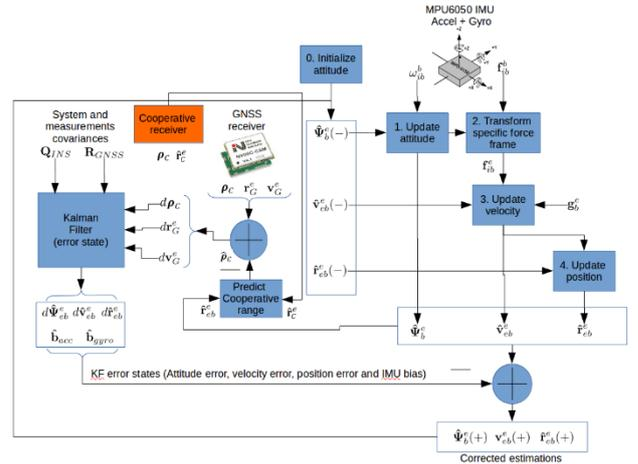
Fig. 7. Hybrid GNSS/INS/UWB fusion algorithm block-diagram.
