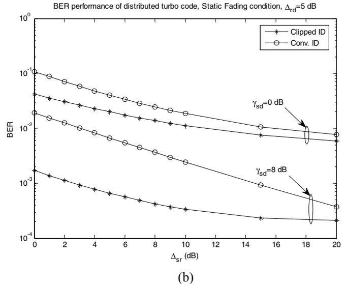
Figure 5, BER performance sensitivity to source-to-relay reliability of the considered cooperative distributed turbo code with conventional and proposed clipped iterative decoders. Results are shown for different SNR conditions  $\gamma_{sd}$  and  $\Delta_{rd}=5$  dB under (a) fast fading, and (b) static fading conditions.
