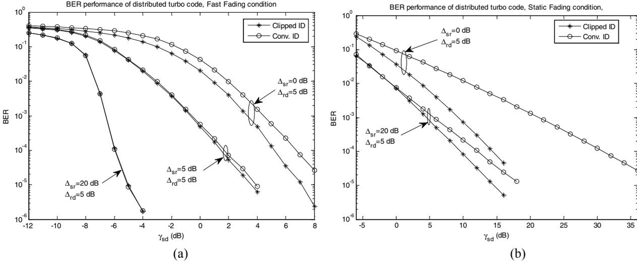
Figure 4, BER performance of the considered cooperative distributed turbo code with conventional and proposed clipped iterative decoders. Results are shown for different SNR offsets  $\Delta_{sr}$  and  $\Delta_{rd}=5$  dB under (a) fast fading, and (b) static fading conditions.
