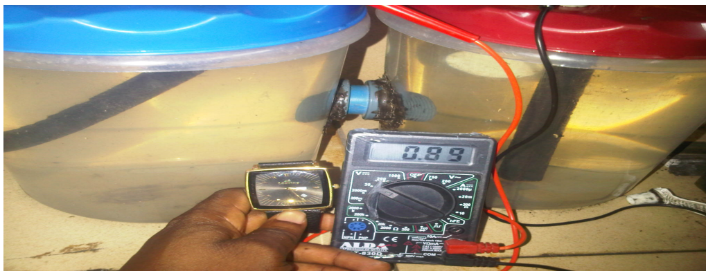
Fig. 4: Photograph showing voltage taken on the 14 th day from cell 1
