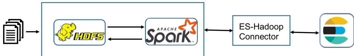
Figure 4.5.3-1: General flow of data transfer from HDFS to ES and vice versa
