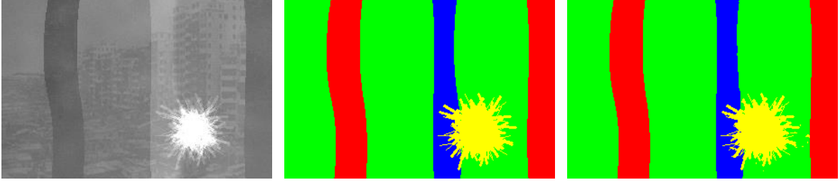
Figure 6: Example for segmentation calculated by the neural network on unseen artificial data. Normalized input range image (left), ground truth segmentation (center), and neural network output (right). Color coding is the same as in Figure 4.
