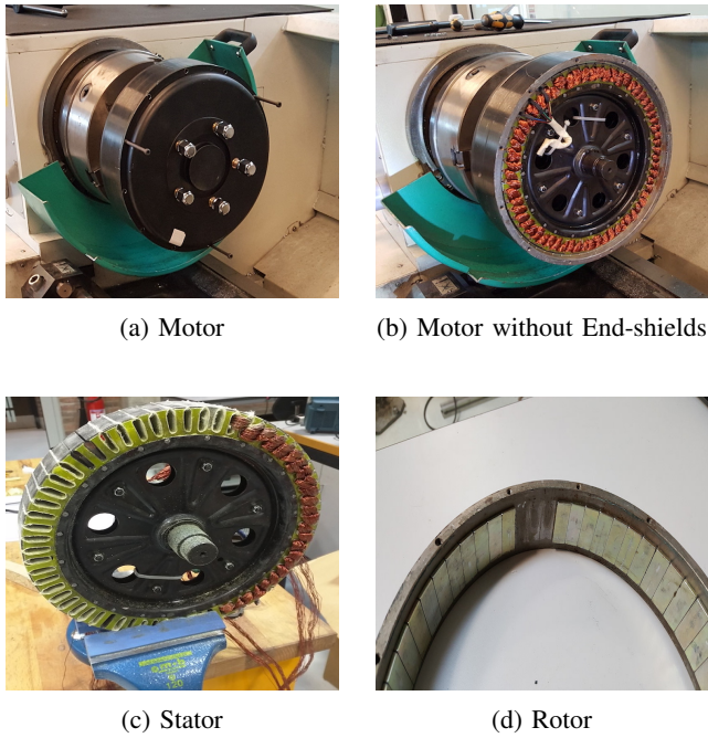
Fig. 3: HUB Motor Disassembly
