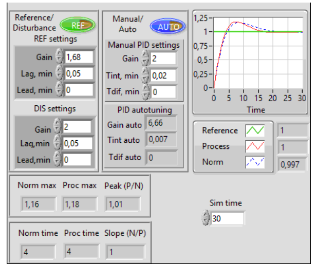
Fig. 6. LabVIEW user interface of the speed control system.
