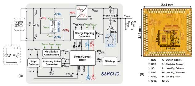
Fig. 1. (a) Synchronized Switch Harvesting on Capacitor-Inductor (SSHCI) interface circuit, and (b) die micrograph of the implemented SSHCI chip.
