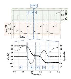
Fig. 3. Measured waveforms of piezoelectric voltage  $V_{PZ}$ , reverse current detector output RCD<sub>0</sub>, and inductor current  $i_{IND}$  during operation phases.
