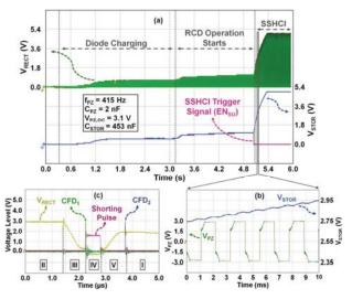
Fig. 7: Measured waveforms of SSHCI circuit illustrating (a) start-up, (b) charging, and (c) control signals generated during voltage flip operations.
