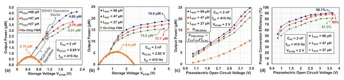
Fig. 8: (a, b) Measured output power by SSHCI circuit compared to on-chip full-bridge rectifier (FBR) with different piezoelectric open circuit voltage levels V<sub>PZ,OC</sub>, and (c) ideal FBR, and (d) power conversion efficiency of the operation. TADIEI
