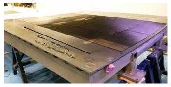
*Figure 8: Setup for ADMP part manufacturing. Carbon fiber material is automatically placed and inspected.*
