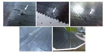
Figure 1: Various kinds of defects, such as wrinkles, early cut tapes, foreign objects (top row), and large gaps (bottom row).
