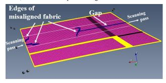
Figure 9: Features representing ply boundaries and gap backprojected onto the surface of manufactured part.
