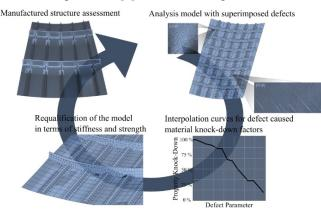
Figure 7: Analysis method to efficiently determine the effects of defects in a composite part [1].
