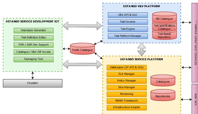
Figure A-3: Overall 5GTANGO architecture [101]
