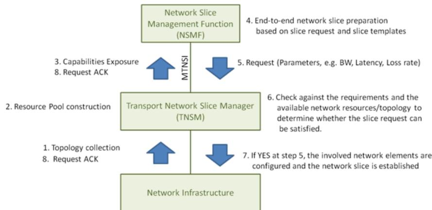
**Figure 4-10: NSMF - TNSM mapping procedures**
