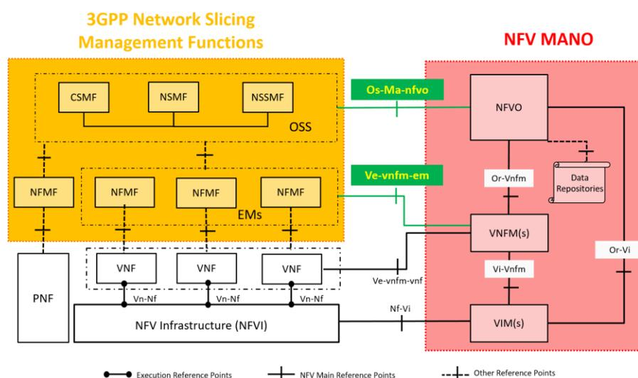
**Figure 2-5: 3GPP network slicing management in NFV framework (adapted from [20])**
