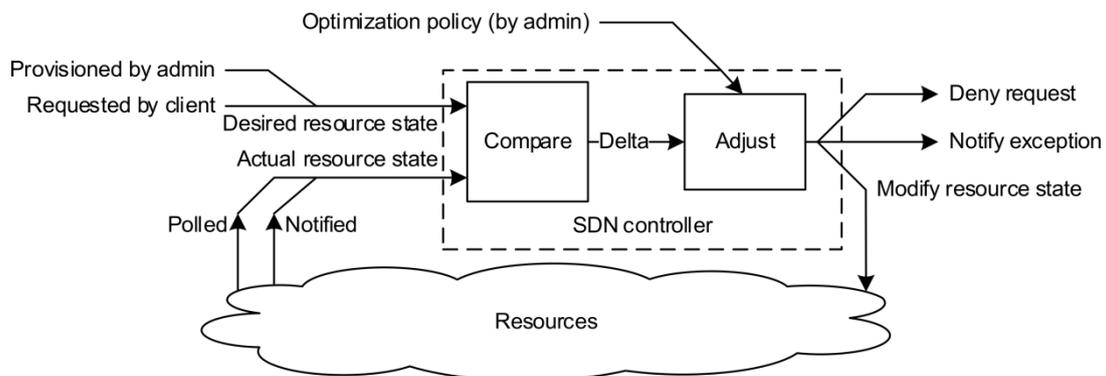
**Figure 5-4: Control as feedback [80]**
