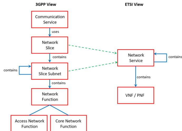
**Figure 2-3: Relating 3GPP and ETSI models in the context of network slicing [20]**
