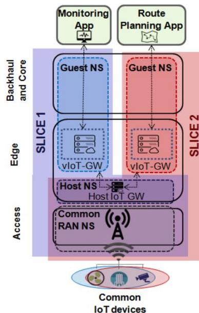
**Figure 6-2: Extended mMTC Slicing Model**
