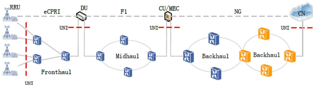
**Figure 4-12: Transport network architecture for independent CU and DU deployment [56]**
