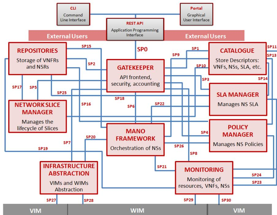
**Figure 2-11: SONATA Service Platform Architecture [36]**
