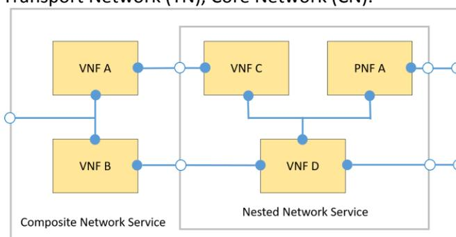
**Figure 2-4: An example of a composite NFV network service (adapted from [22])**
