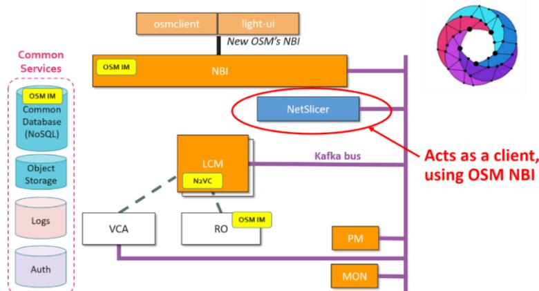
**Figure A-5: Integration of 5GTANGO Slice Manager into OSM Release 5**
