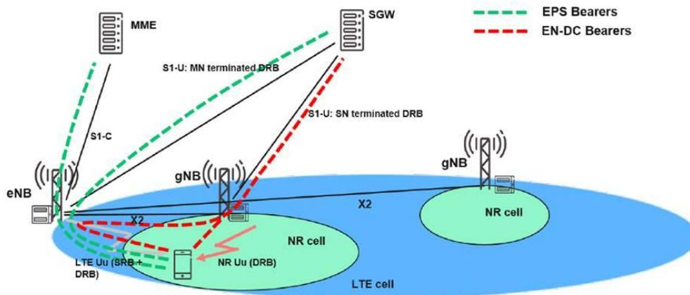
**Figure 4-3: Conceptual Architecture for EPS with EN-DC (Option 3x)**
