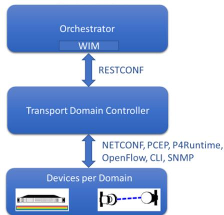
**Figure 4-15: Transport SDN controller NBIs and SBIs**
