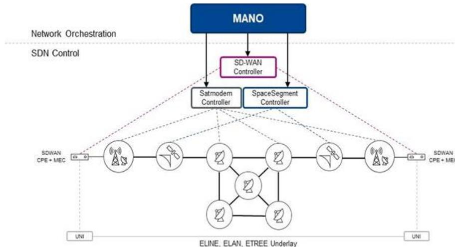
**Figure 4-21: Distributed SDN Controller Architecture [77]**
