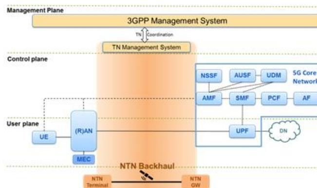
**Figure 4-17: Satellite transport network based on 3GPP system specifications [75]**
