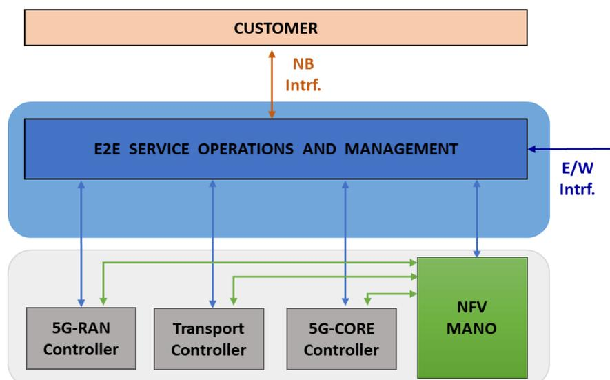
**Figure 3-1: Architectural Components for the slice life cycle management and orchestration**
