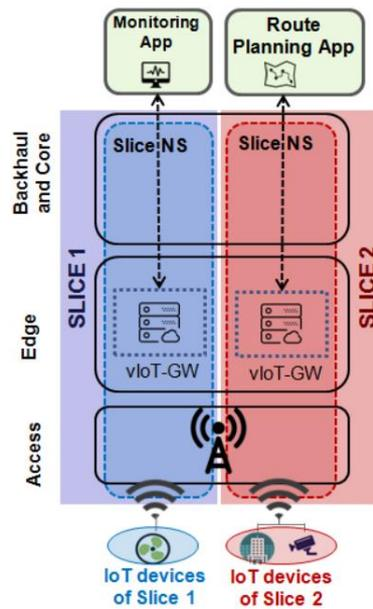
**Figure 6-1: Baseline mMTC Slicing Model**
