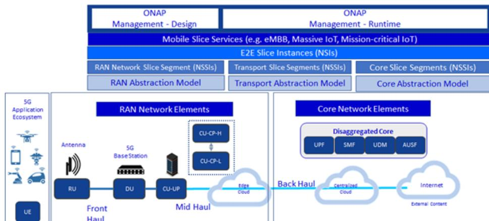
Figure 2-12: 5G network slice - network architecture with ONAP management [38]
