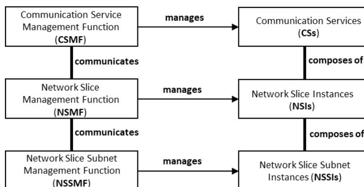
**Figure 2-2: 3GPP defined Network Slicing management functions and managed entities**
