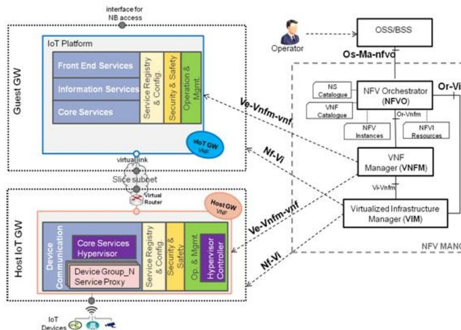
**Figure 6-3: Interfaces for mMTC slice lifecycle management**
