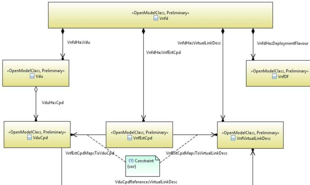
Figure 5-9: VNFD High-level structure
