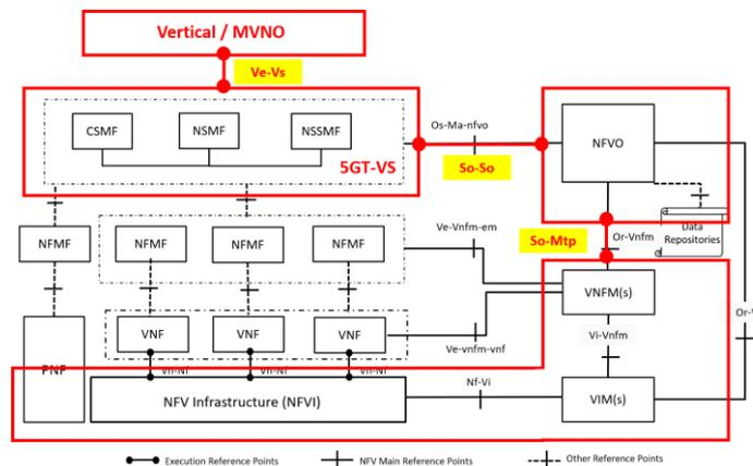
**Figure A-2: Mapping 5G-TRANSFORMER architecture into 3GPP/NFV network slicing framework**
