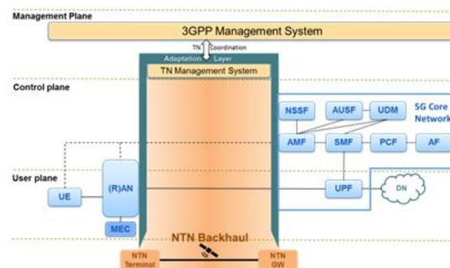
**Figure 4-18: Satellite transport network not based on 3GPP system specifications [75]**
