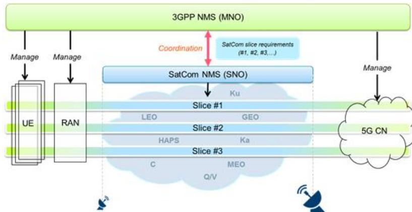
**Figure 4-19: Slicing management in satellite transport network [76]**
