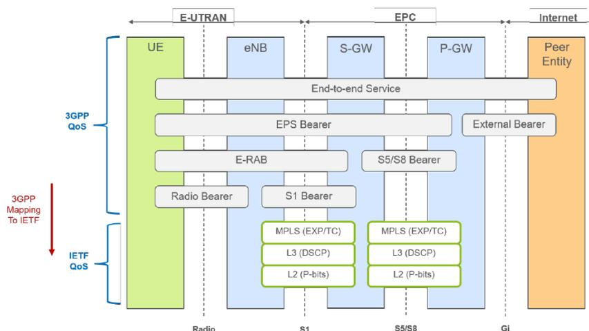
**Figure 4-2: E2E QoS design uses a blend of the 3GPP and IETF QoS architectures**
