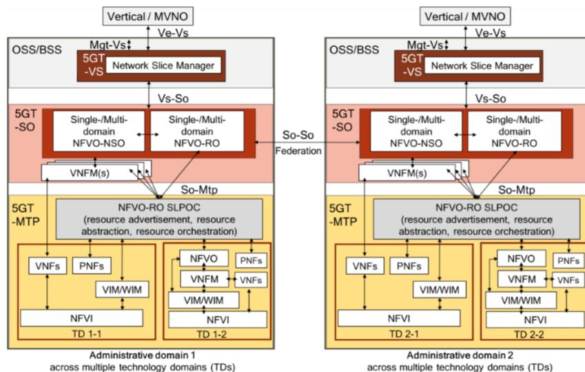
**Figure A-1: 5G-TRANSFORMER system architecture [97]**
