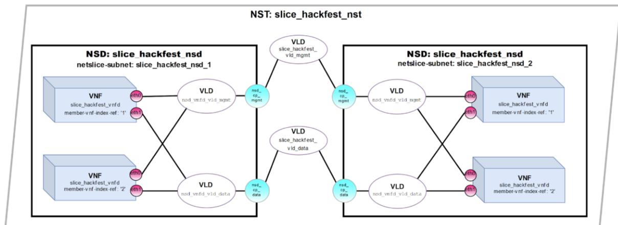
Figure 5-11: NST information model for OSM release 5, from OSM 5<sup>th</sup> Hackfest
