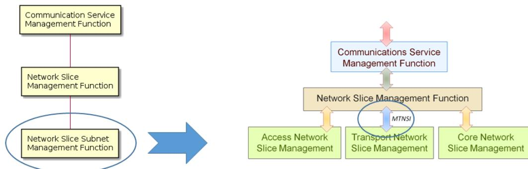
**Figure 4-9: 3GPP network slice management functions and BBF focus**
