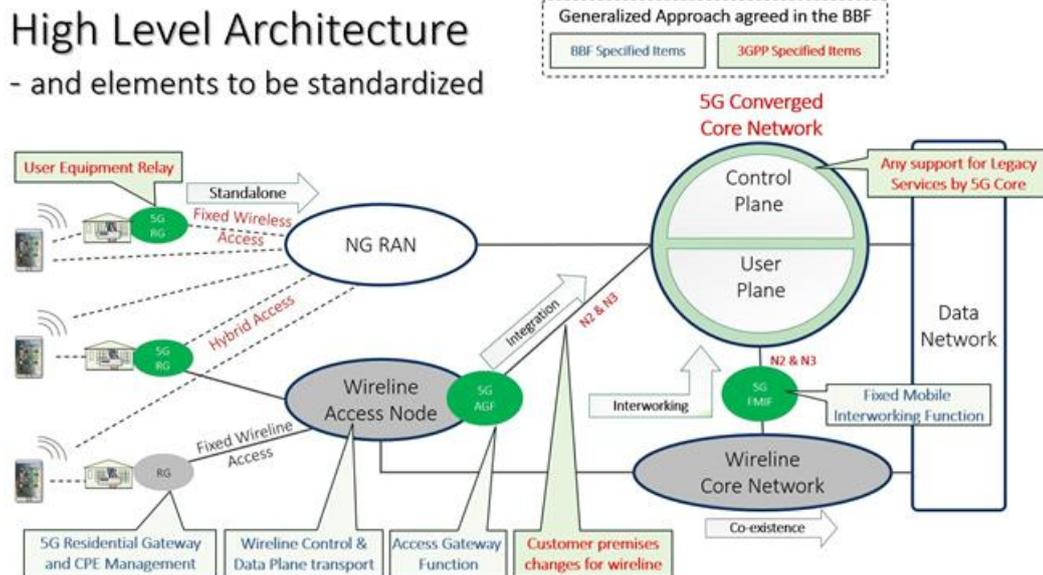
**Figure 4-6: BBF 5G FMC architecture and elements to be standardized [55]**
