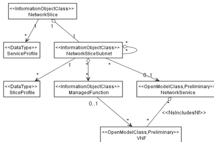
**Figure 2-1: UML diagram showing the network slice, network slice subnet and NF hierarchies**
