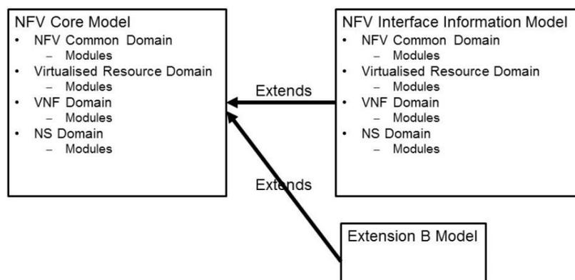
Figure 5-8: NFV Core Model extensions
