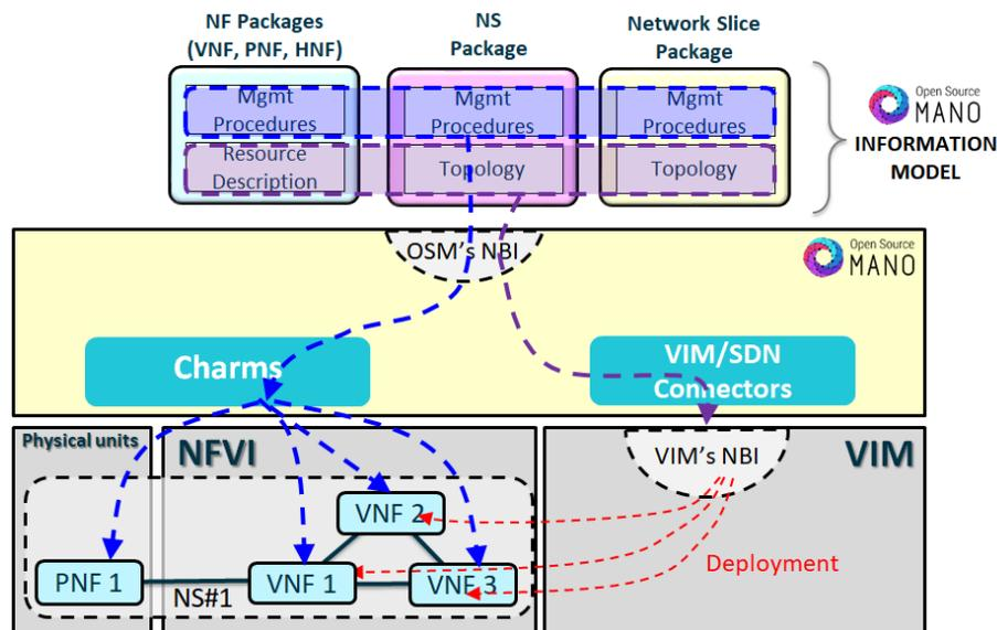
Figure 2-10: IM and NS operation via NBI [35]
