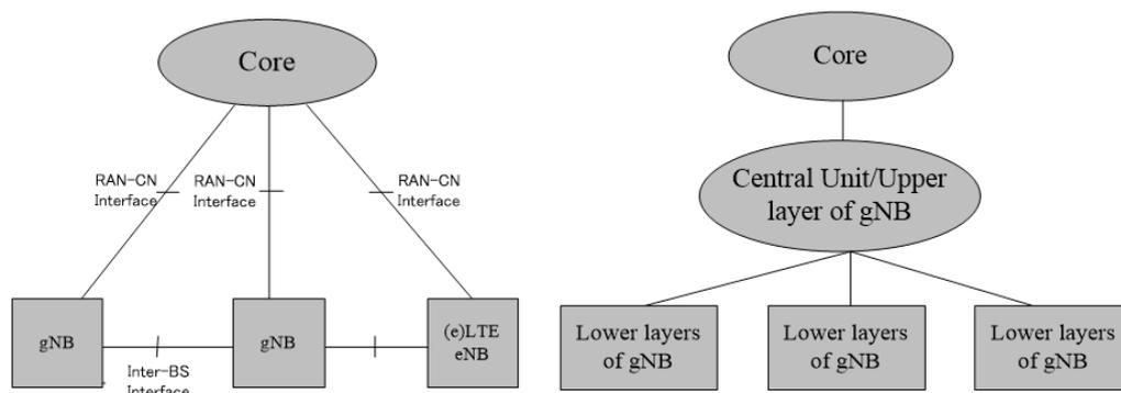
**Figure 4-11: Non-centralized vs. centralized RAN deployment [57]**
