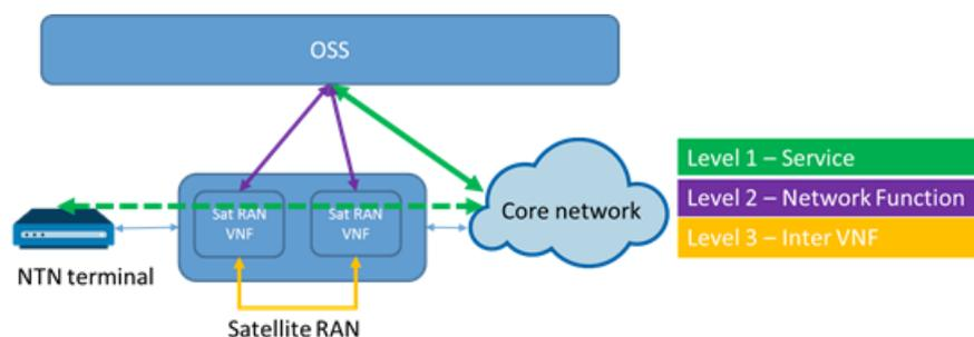
**Figure 4-22: Enabler for network slicing in a satellite communication system [78]**
