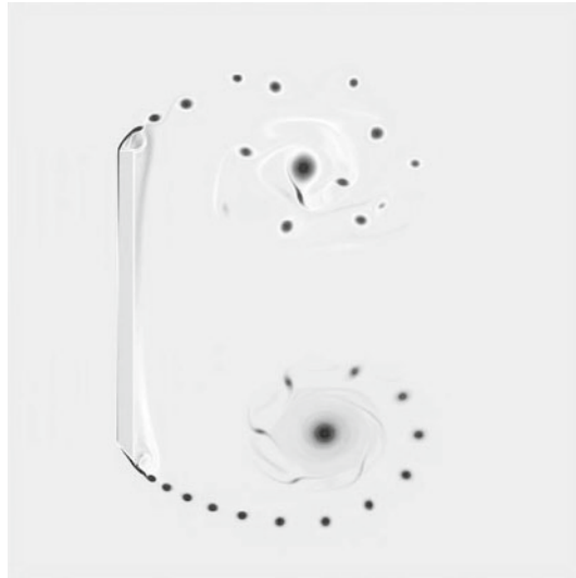
Fig. 3 Vorticity field (zoom) at t = 1.4 for the impulsively started plate at Re = 9500
