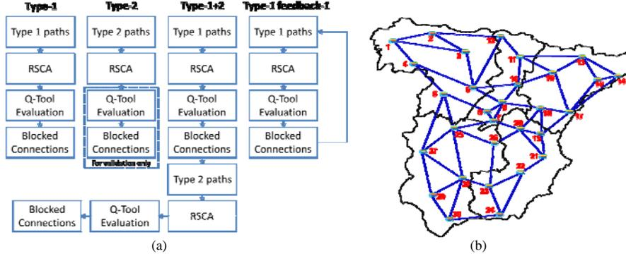
Figure 1. (a) Flowcharts of the proposed algorithms, (b) Topology of the Telefonica network [2].
