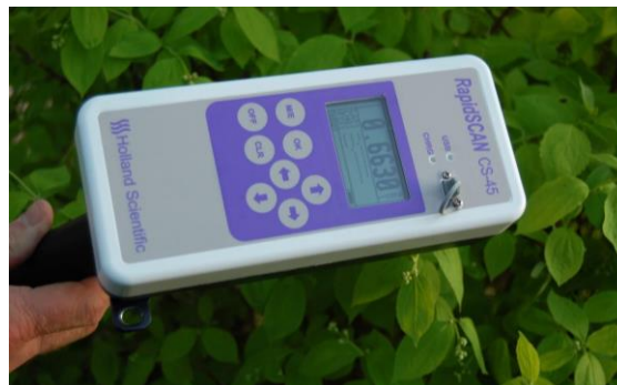
Figure 5: Crop Circle RapidSCAN AC-45 handheld reflectance sensor
