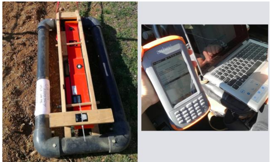
Figure1: EM38-MK2 (left) and Archer Data logger (right)
