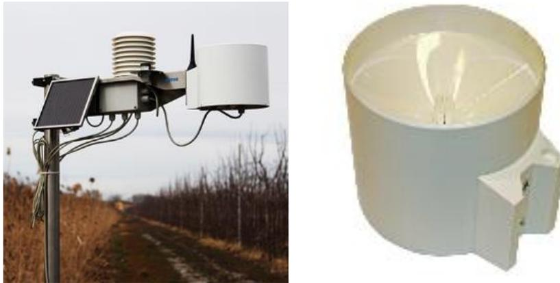
Figure 5: Sensor & Weather Station (left) and Rain Gauge Module (right)
