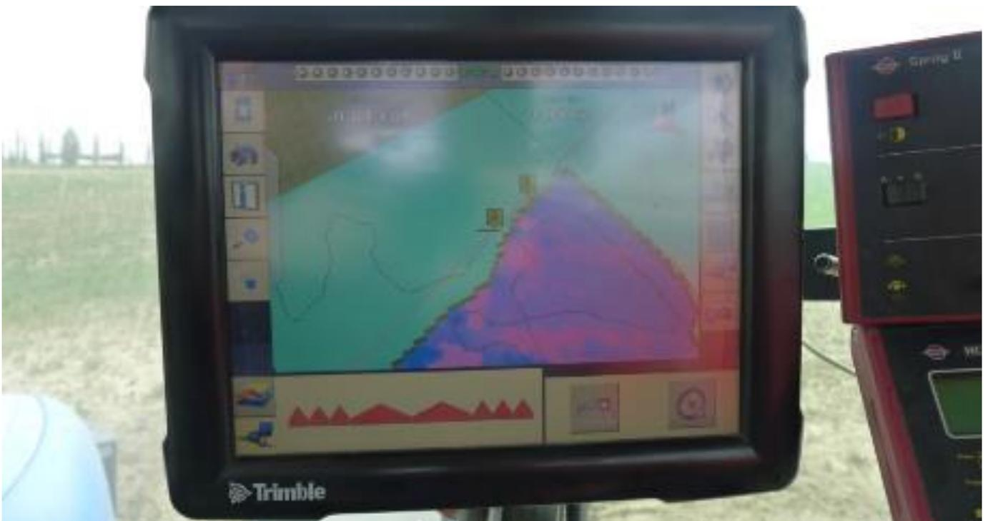
Figure 18 Import of a prescription map on a Trimble VR computer.
