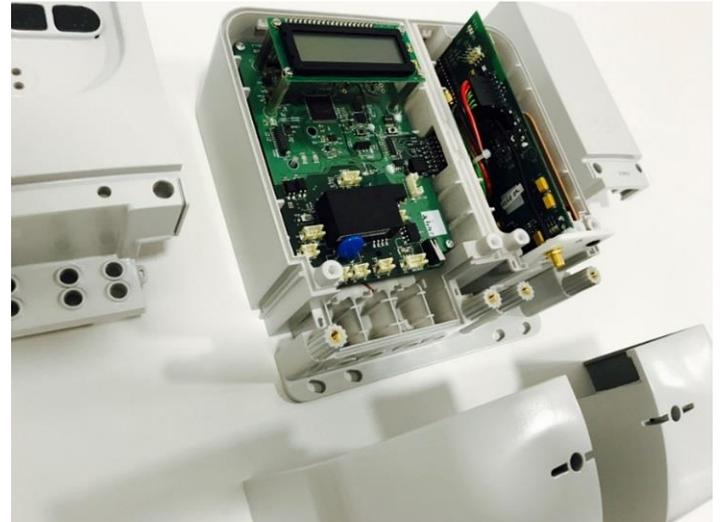
Fig. 2. SLAM: Next generation smart meters by NOBEL GRID
