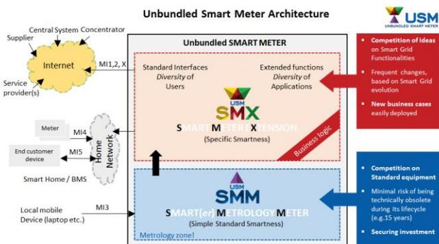
Fig. 1. Unbundled Smart Meter architecture
