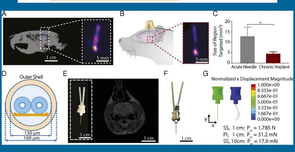
Chronic MiNDS probes for focal deep-brain interfacing. (*A*) PET/computed tomography (PET/CT) scans of rat head following 2-µL acute injection of Cu-64 in vivo. (*B*) Illustration of implanted short, minimally invasive drug delivery system (S-MiNDS) probe in a rat. (*Inset*) PET images of 2-µL infusion of Cu-64 through chronically implanted probe. (*C*) Size of brain region targeted using infusion through acutely inserted needle and chronic implant.
