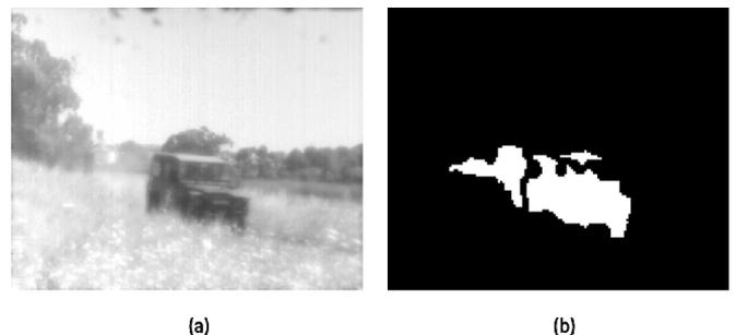
Fig. 2. Example of sensor outdoor test. a) QVGA grayscale image; b) Quarter-QVGA event bitmap after the chip-embedded erosion filter.
