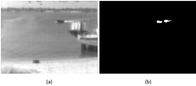
Fig. 5. Example of the sensor operation. a) QVGA grayscale image; b) quarter QVGA hot-pixel bitmap after erosion.
