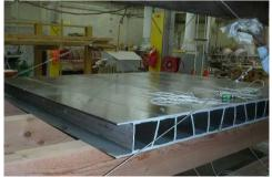
Fig. 1. GFRP deck panel
