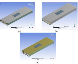
Fig. 3. Cross section of all GFRP deck panels – (a) Rectangular GFRP deck panel with L/D ratio 2 (b) Trapezoidal GFRP deck panel with L/D ratio 2 (c) Elliptical GFRP deck panel with L/D ratio 2
