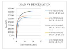
Fig. 9. Load deformation behavior of conventional deck panel along the length and across the width of deck
