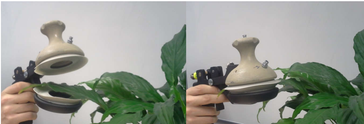
Figure 2-9: Sample taking directly on the leaf.
