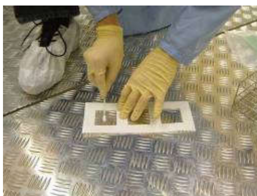
Figure 2-15: Sample Taking of a Surface.
