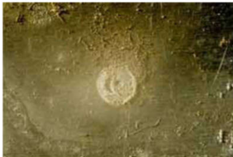
A generated hole in aluminum by a fungus on the MIR
