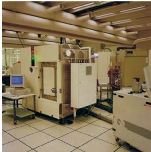
Fig. 13. ALD reactor F-1000 by Microchemistry Ltd. for coating big batches of 500 mm × 500 mm substrates. Photo from Suntola's collections; published with permission of Tuomo Suntola (private collection).
