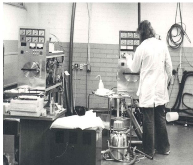
Fig. 4. Arto Pakkala operates reactors used for early ALE-EL prototypes. Photo from Suntola's collections; published with permission of Tuomo Suntola (private collection).
