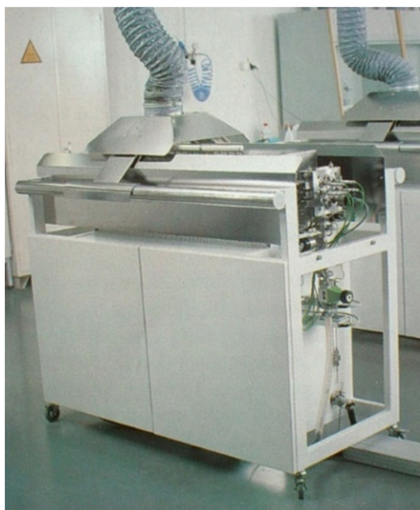
Fig. 10. The F-120 reactor. The heavy bars on each side of the reactor were meant to let the researcher lean and ponder while looking at the progress of the process. Photo from Suntola's collections; published with permission of Tuomo Suntola (private collection).
