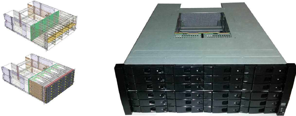
Figure 4. Data storage and switch enclosure for 19" data center racks based on 4U24 form factor
