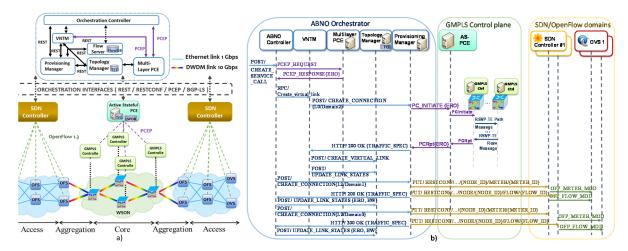
Fig. 1: a) Reference SDN orchestration architecture; b) Multilayer E2E service orchestration workflow.
