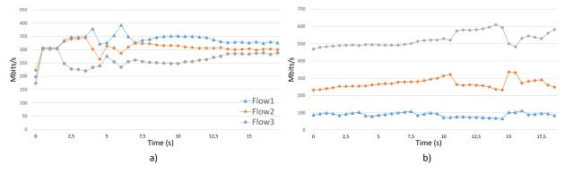
Fig. 4: Per-flow bandwidth limitation; a) IO graph OF Switch output\_port without meter limitation; b) IO graph OF Switch output\_port throughput with 600, 300 and100 Mbps meter limitation.
