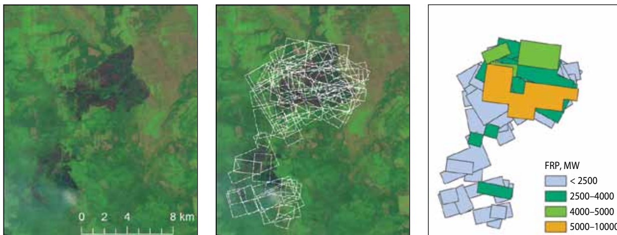
Fig. 1. Series of high-temperature events (white polygons) detected by TERRA/Modis over wildfire and the result of FRP classification. Landsat image of active fire is in the background
