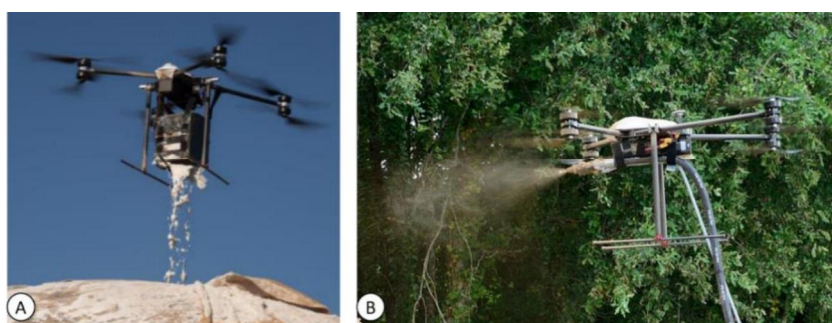
Figure 3: A) Drone carrying container with clay mix (from [2]) B) Drone with pipe connected to matter mixer and water
