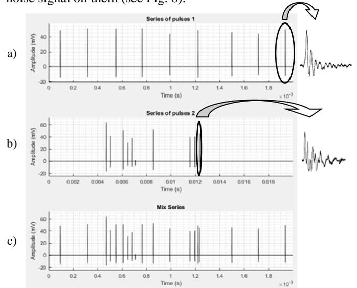
Fig. 5. Synthetic generation of analogue PD time series. a) Corona effect, b) surface defect and c) simultaneous generation of the corona effect and the surface defect.
