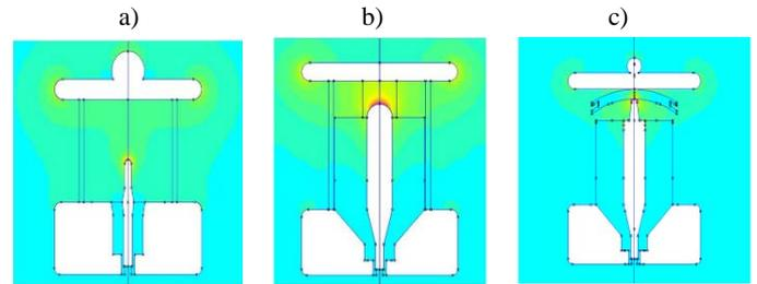
Fig. 3. Layout of the test cells and electrical field distribution calculated by means of FEMM. a) Corona effect in air, b) internal defect in polyethylene and c) surface defect in glass.
