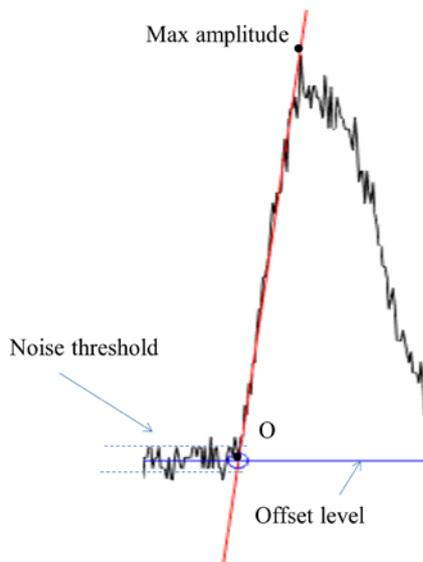
Fig. 4. Detection of the PD pulses and determination of their origin for the final digitalisation.
