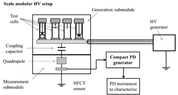
Fig. 2. Layout of the scale modular HV setup developed for the generation and recording of the reference PD time series.
