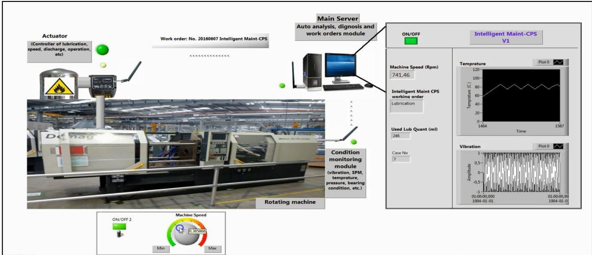
Fig. 2. Front panel of the Intelligent Maint-CPS simulation
