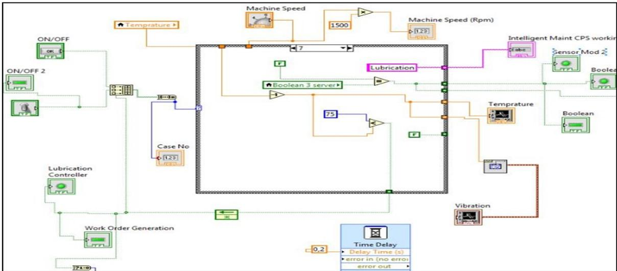
Fig. 3. Block diagram panel of the Intelligent CPS-Maint simulation.
