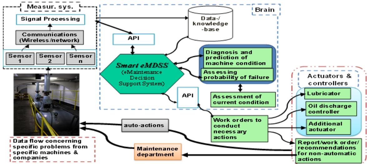
Fig.1. Intelligent CPS - Maint; data flow, diagnoses, prediction, assessments and self-healing actions
