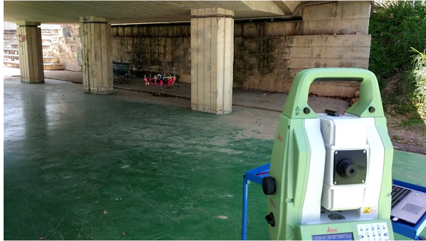
Fig. 7. Total Station taking measurements for odometry position under one of the bridges.
