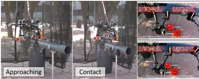
Figure 10. Approaching (left) and contact force control (right) phases seen from the onboard camera. The position of the left/right arms and the target contact point are measured with ARUCO tags.
