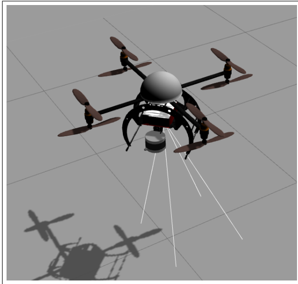
Fig. 3 The UAS model used in simulation with its VLP-16 LIDAR in front.
