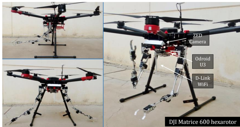
Fig. 7. Three views of the dual arm aerial manipulation system integrated in the DJI Matrice 600 hexarotor.
