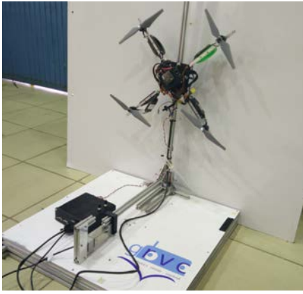
Fig.8. Test stand with quadrotor during experiments.
