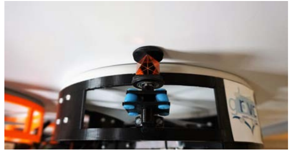
Fig.16. Quadrotor in contact with the ceiling while the prism is in contact.
