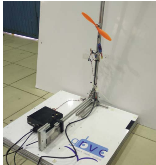
Fig. 3. Test stand with single rotor during experiments
