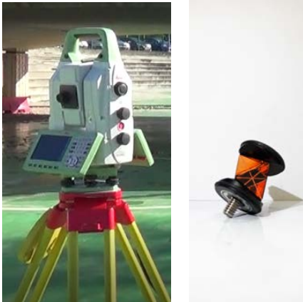
Fig.14. Leica total station and reflector prism to be mounted on the UAV
