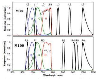
Figure 3. Normalized MSL/Mastcam system-level spectral response profiles for the left eye M-34 camera (top panel) and the right eye M-100 camera (bottom panel) [1].
