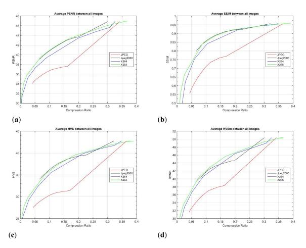
Figure 9. PCA-6: Comparison of different algorithms for 20 right images shown in Figure 5: (a) PSNR in dB for right images; (b) SSIM for right images; (c) HVS in dB for right images; (d) HVSm in dB for right images.
