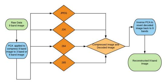
Figure 1. Proposed 2-step compression scheme for Mastcam images.
