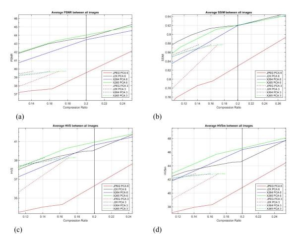
Figure 13. Comparison of PCA-3 and PCA-6 for right Mastcam images. Region of interest: compression ratio of 0.2: (a) PSNR in dB for right images; (b) SSIM for right images; (c) HVS in dB for right images; (d) HVSm in dB for right images.
