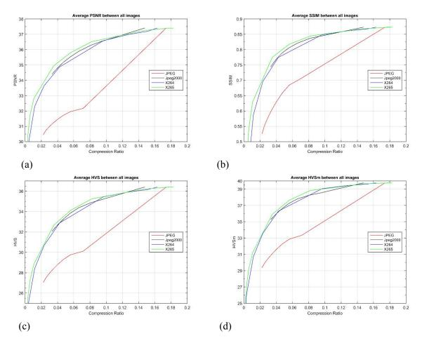
Figure 6. PCA-3: Comparison of different algorithms for 20 left Mastcam mages shown in Figure 4: (a) PSNR in dB for left images; (b) SSIM for left images; (c) HVS in dB for left images; (d) HVSm in dB for left images.
