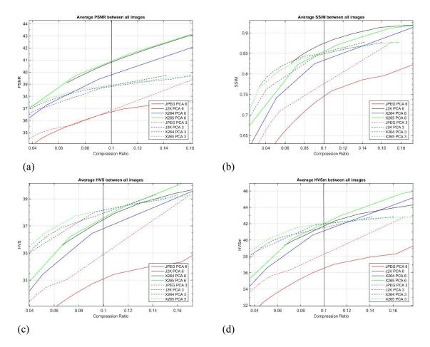
Figure 11. Comparison of PCA-3 and PCA-6 for right Mastcam images. Region of interest: compression ratio of 0.1: (a) PSNR in dB for right images; (b) SSIM for right images; (c) HVS in dB for right images; (d) HVSm in dB for right images
