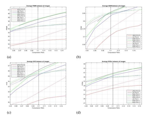
Figure 10. Comparison of PCA-3 and PCA-6 for left Mastcam images. Region of interest: compression ratio of 0.1: (a) PSNR in dB for left images; (b) SSIM for left images; (c) HVS in dB for left images; (d) HVSm in dB for left images.
