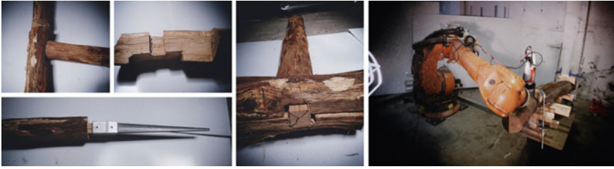
Fig. 11 Fabrication of 1:1 scale prototypes of timber joints with a chainsaw-equipped robot/Robotic Fabrication Workshop @ IaaC|2013. © Vicente Gasco
