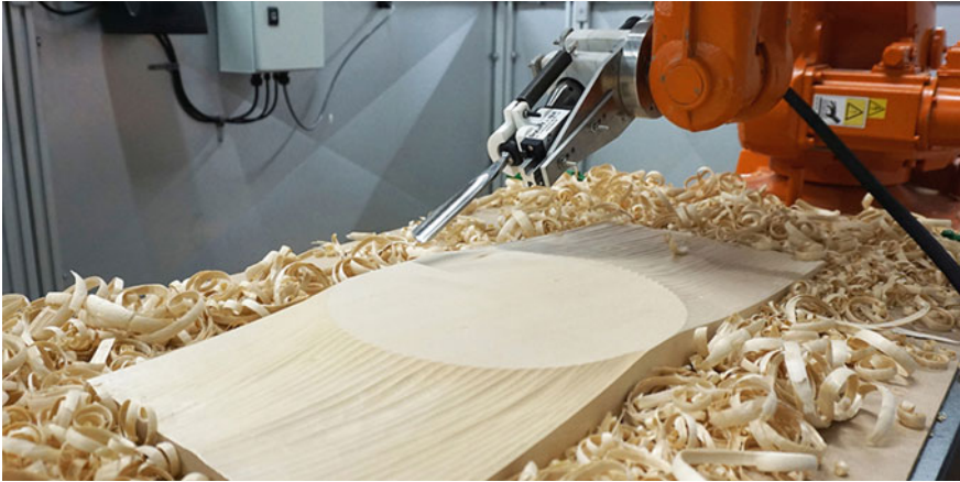
Fig. 16 During the fabrication stage, the robotic toolpath is optimized to match the original design intention with tool affordances and material properties, such as the wood grain directionality. © Giulio Brugnaro
