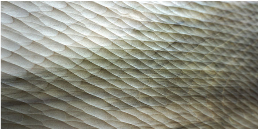
Fig. 17 The trained system could be used to predict combinations of multiple cuts to generate specific patterns on the carved surfaces. © Giulio Brugnaro
