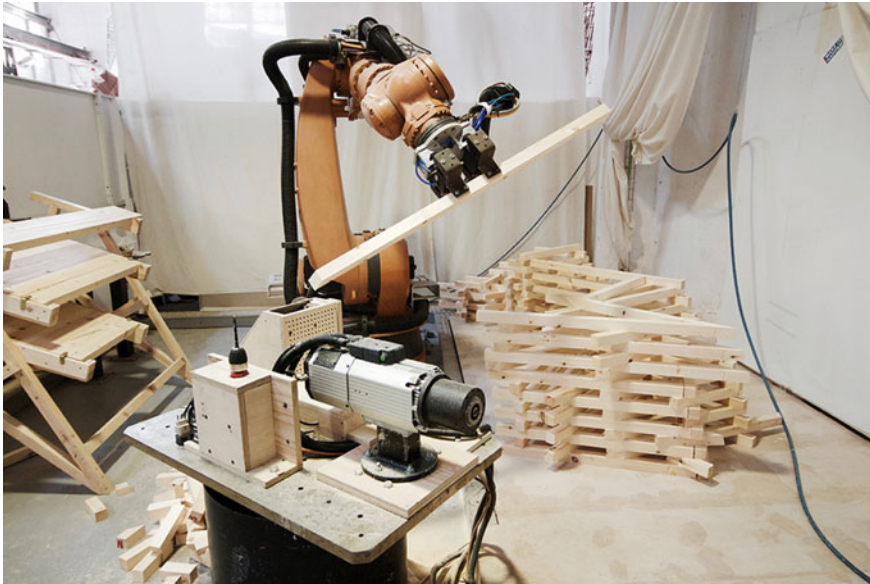
Fig. 5 Digital Urban Orchard 2016: robotic fabrication process. © Andrea Quartara
