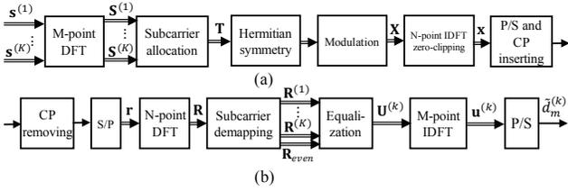
Fig. 1. Block diagram of the transmitter and the receiver for the  $k$ th user in a downlink VLC system based on SC-FDMA.
