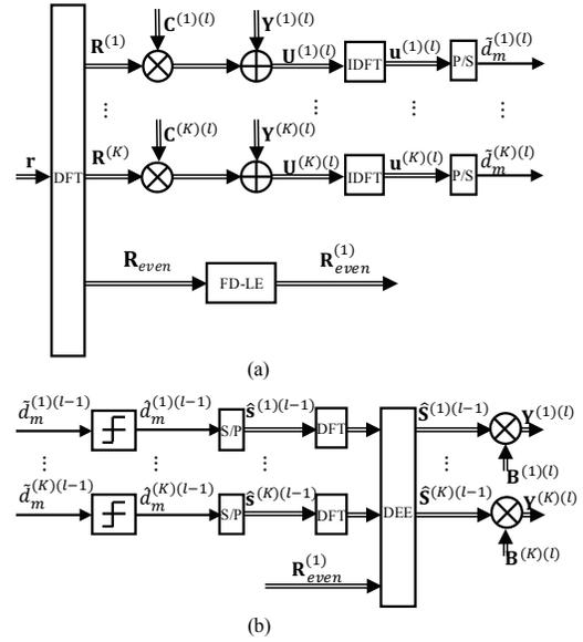
Fig. 2. Block diagram of the proposed FD-DFE structure.
