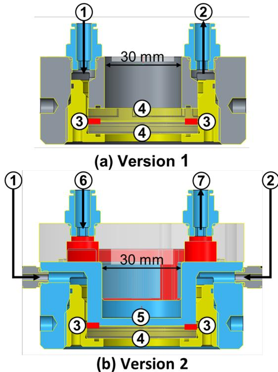
**Figure 2.** Two versions of the calibration tool. The numbered elements are discussed in the text. Typically, the direction of laser irradiation and fluorescence detection are from the bottom.
