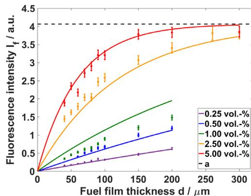
**Figure 6.** Variation of liquid film thickness for different concentrations of toluene in iso-octane. Solid lines represent the global fit to the Lambert-Beer (equation (4)).
