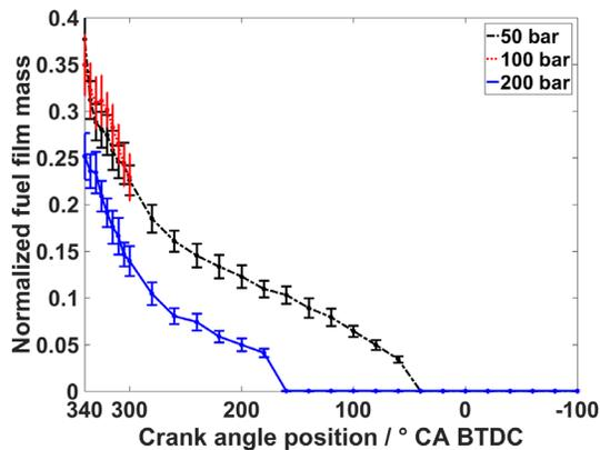
**Figure 15.** Fuel-film mass as a fraction of the injected mass as a function of crank angle during compression and early expansion.
