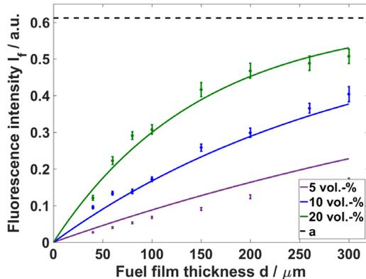
**Figure 7.** Variation of liquid film thickness for different concentrations of 3-pentanone in iso-octane. Solid lines represent the global fit to the Lambert-Beer (equation (4)). The values for fluorescence signal (on the y-axis) are consistent with those in Figure 6.
