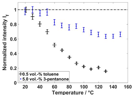
**Figure 9.** Temperature dependencies of toluene and 3-pentanone fluorescence at 14 bar. Intensities are normalized by values at room temperature.
