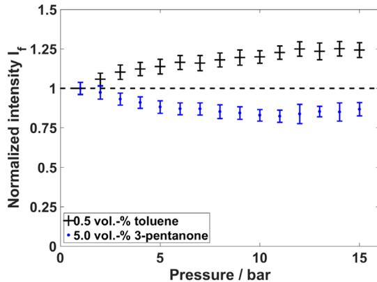
**Figure 8.** Pressure dependencies of toluene and 3-pentanone fluorescence at 20°C. Intensities are normalized by the values at ambient pressure.
