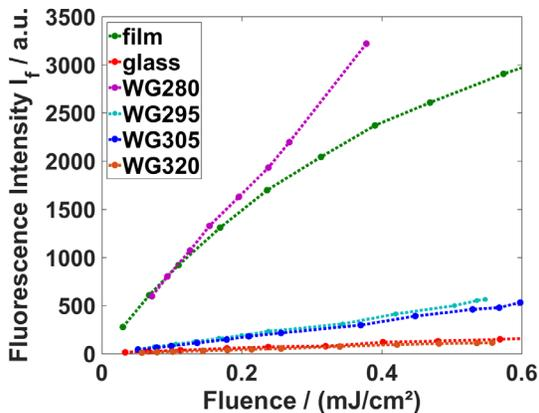
**Figure 4.** Fluorescence intensities from the flat-field material candidates as a function of laser fluence.
