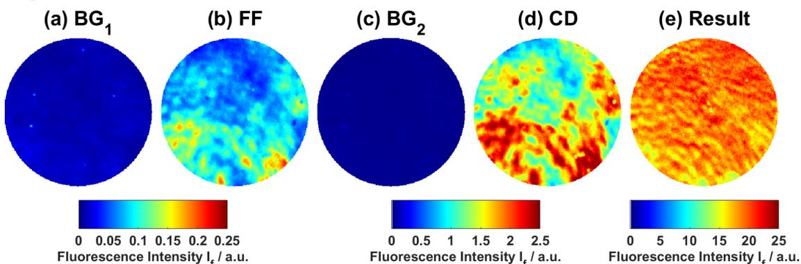
**Figure 5.** Post-Processing for a film of iso-octane/toluene-mixture: (a) Background for the flat-field: empty measurement volume, (b) flat-field, (c) Background 2: calibration device filled with iso-octane (d) Film image: calibration device filled with toluene and iso-octane. (e) Result of the post-processing. Fluorescence intensity is given in arbitrary but consistent units.
