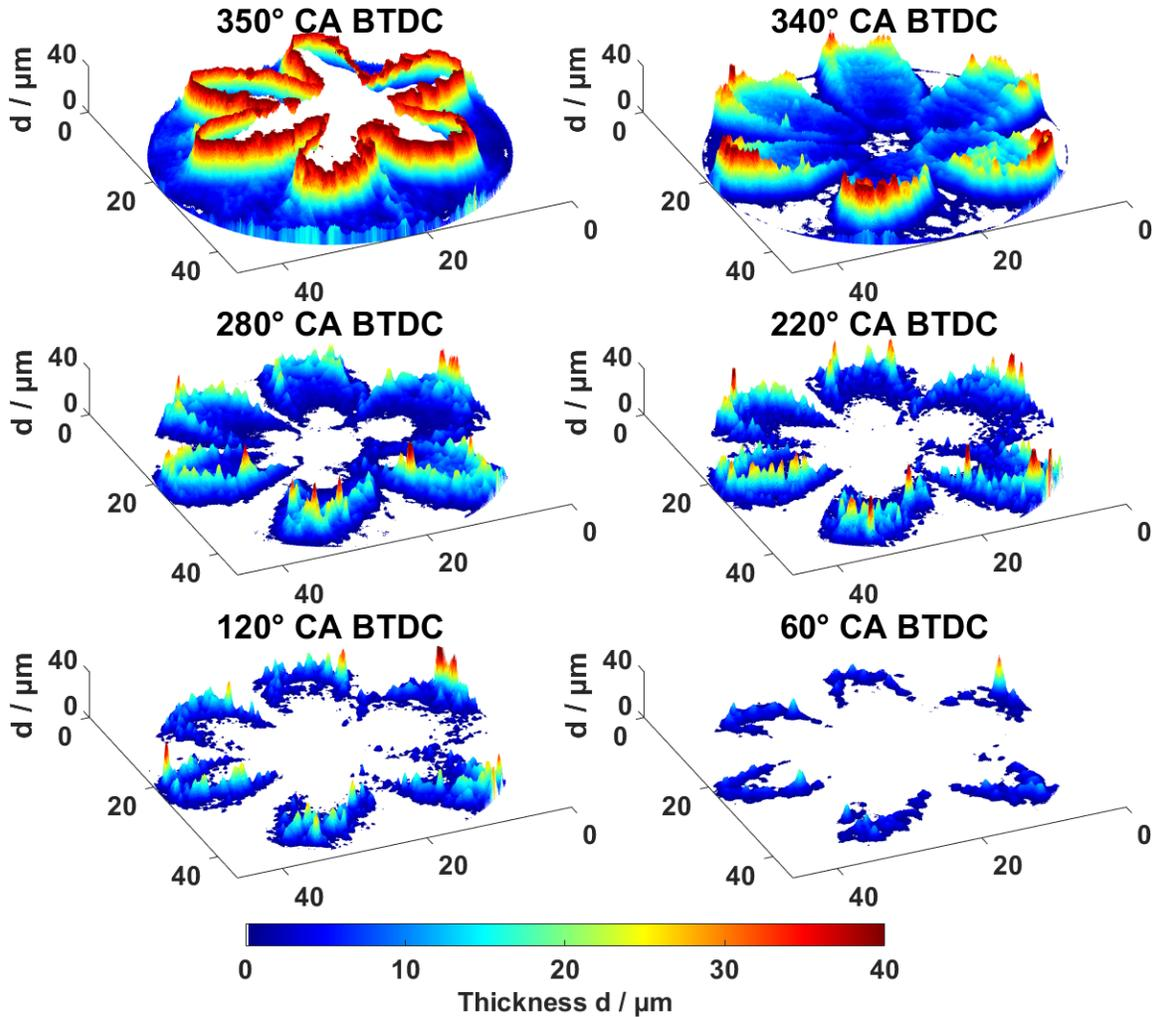
**Figure 14.** Crank-angle series of LIF images converted to fuel-film thickness on the piston top as a function for injection with 50bar. Note that at 350° CA BTDC the LIF signal comes partly from the spray, not only the film, as discussed in the text.
