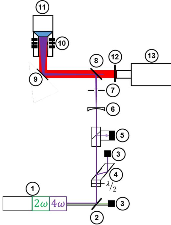
**Figure 1.** Optics and beam path in the experiments. The numbered elements are discussed in the text.
