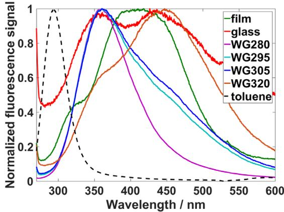
**Figure 3.** Fluorescence spectra from the flat-field material candidates upon excitation at 266 nm.
