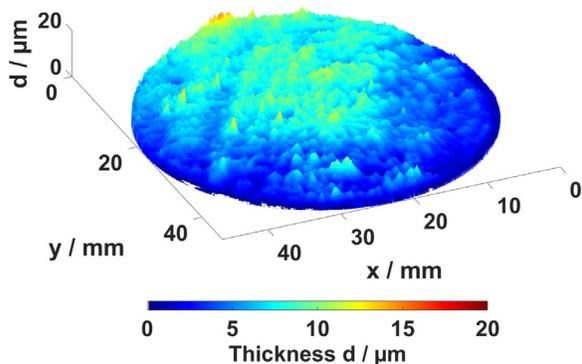
**Figure 12.** Equivalent liquid film thickness corresponding to LIF from the gas phase with PFI in nitrogen. Image timing:  $300^\circ$  CA BTDC.
