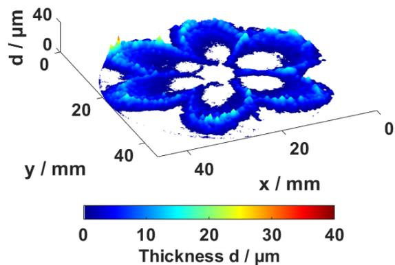
**Figure 13.** Fuel-film thickness on the piston surface for different injection pressures (image timing:  $300^\circ$  CA BTDC).
