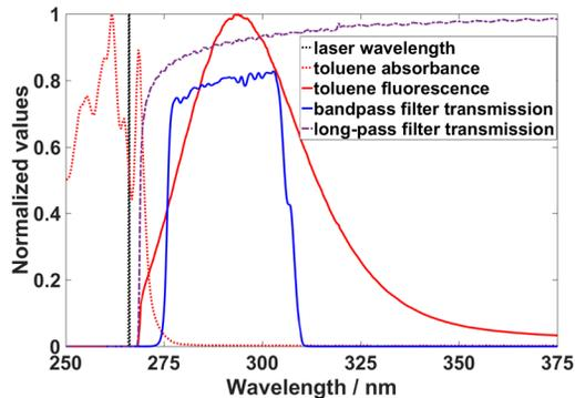
**Figure 10** Transmission spectrum of the detection filter in relation to the fluorescence and absorption spectra of toluene (filter transmission data from data sheets [39, 40]).
