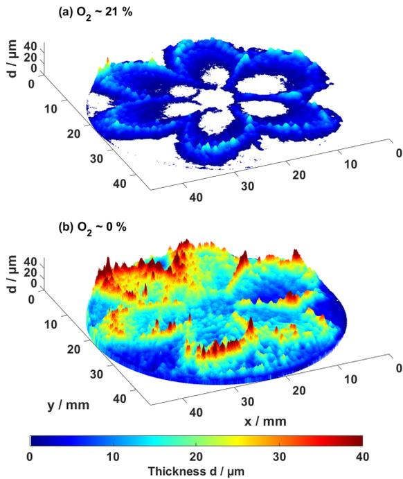
**Figure 11.** Measured fuel-film thickness on the piston surface at  $300^\circ$  CA BTDC for air (top) and nitrogen (bottom) as a bulk gas.
