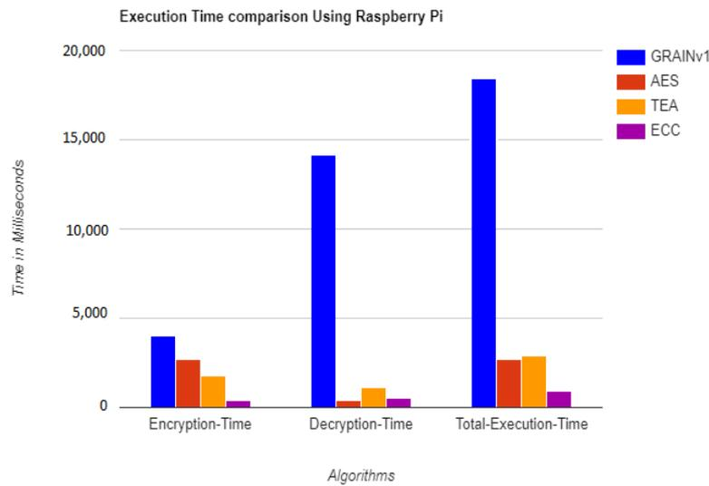
Fig. 8. Comparison of Execution time using Raspberry Pi
