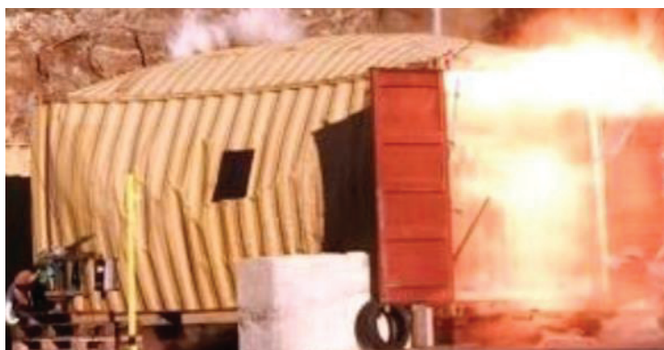
Figure 3. Wall distortion of 20-foot ISO container during vented explosion as captured in an instantaneous image (from Skjold et al., 2017a)
